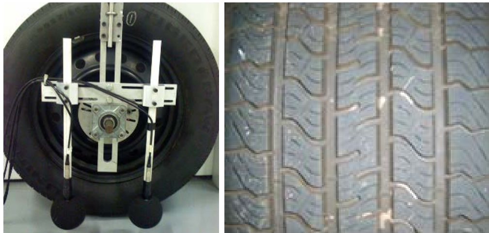
Figure 20. Onboard sound intensity probe and tire tread of the SRTT.
