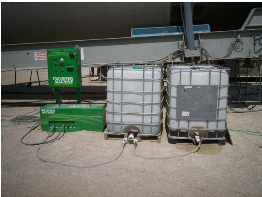
Figure 18. Photo. Foaming system, water added at 1.75 percent of binder. (courtesy: Wyoming DOT)
