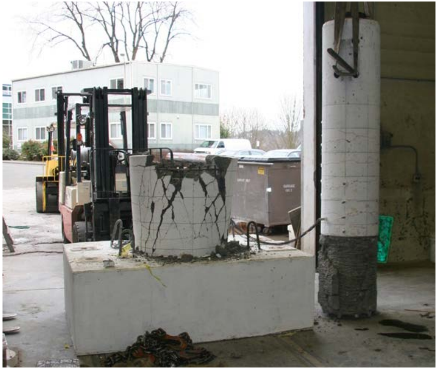
Figure 39. Photo. Specimen DS-2 after testing.
