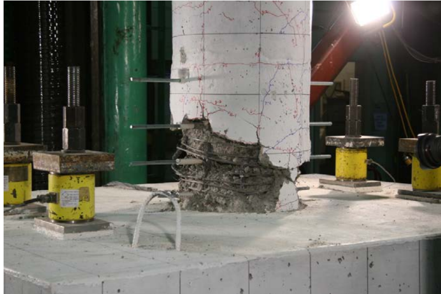
Figure 27. Photo. Specimen SF-2 after completion of cyclic testing.
