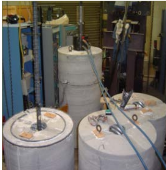
Figure 9. Photo. Test setup for large-bar anchorage testing.
