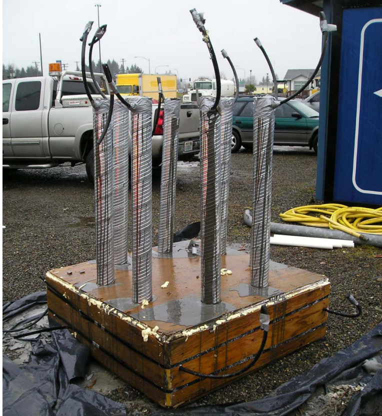
Figure 44. Photo. Mock-up of the grouted joint.
