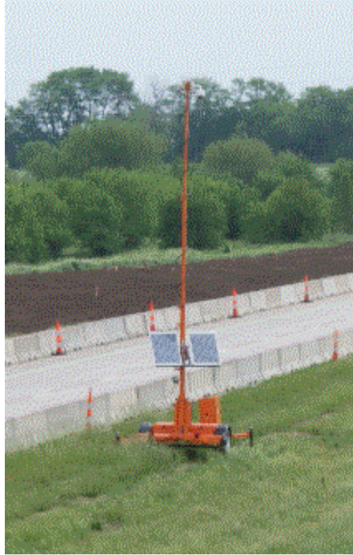
Figure 5. Photo. CCTV trailer.
