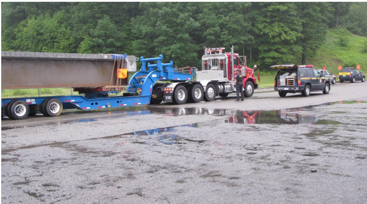
Figure 14. Photo. Transportation of PMSE units to staging area.
