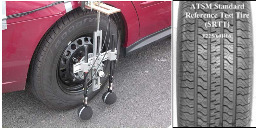
Figure 48. Photo. OBSI dual probe system and the SRTT (source: NCAT).
