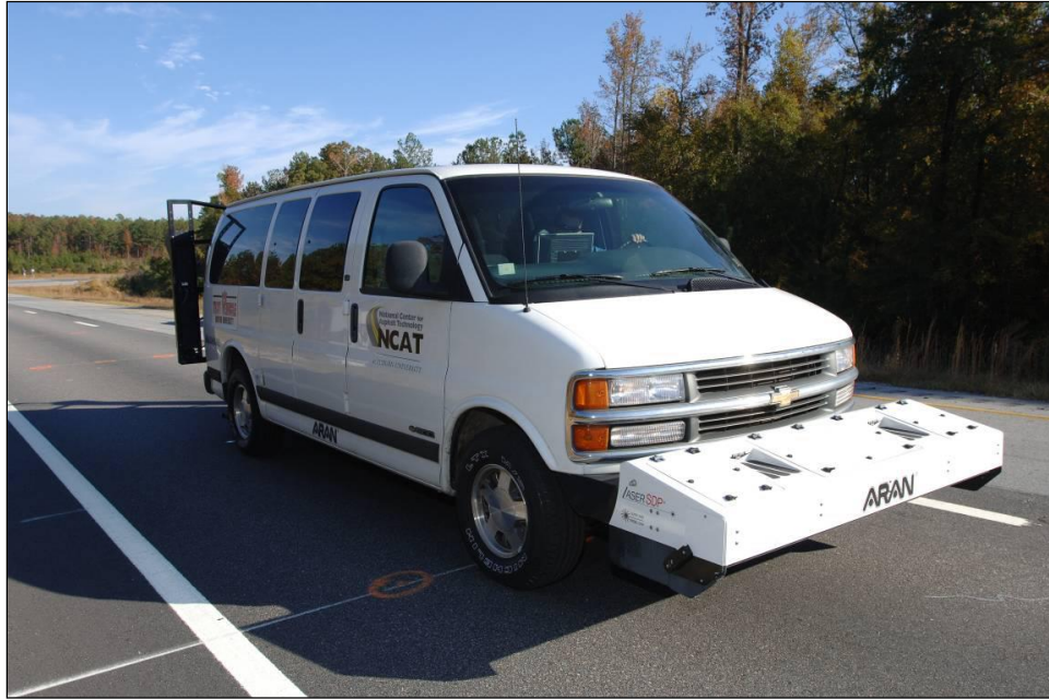
Figure 53. Photo. Auburn University ARAN van. (source: NCAT).
