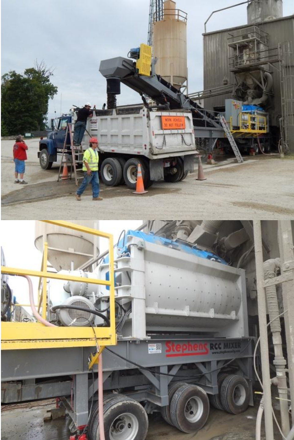
Figure 6. Photos. RCC pugmill integrated with an existing ready mix concrete plant.
