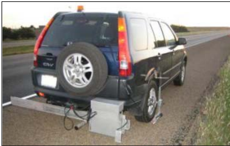
Figure 23. High-speed inertial profiler mounted behind the test vehicle.
