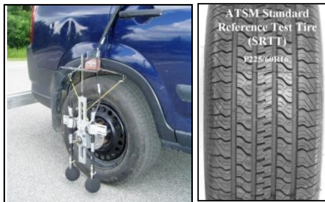
Figure 19. OBSI dual probe system and the SRTT.
