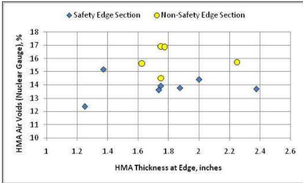
Figure 14. Comparison of HMA thickness at the edge of the mat and HMA air voids.
