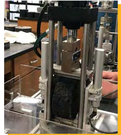
Image Source: FHWA Load frame performing IDEAL-CT
