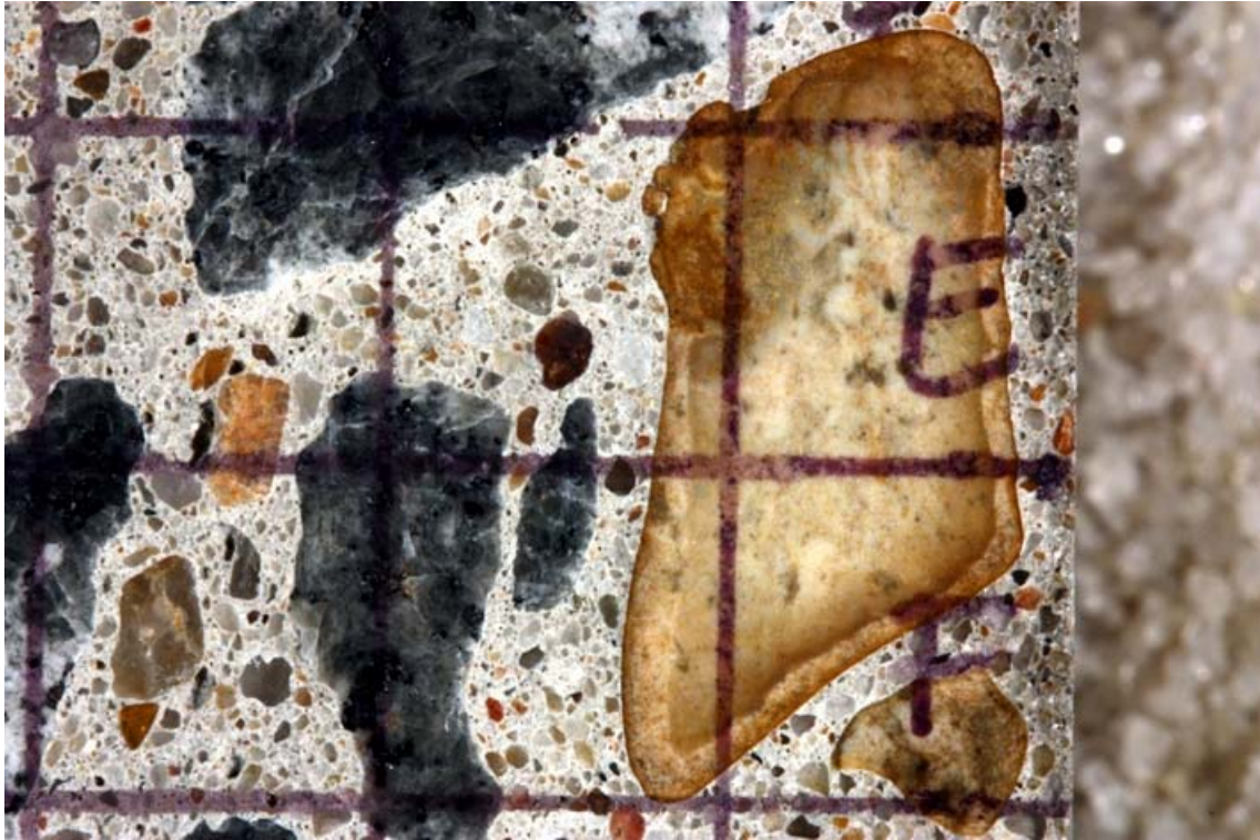
Figure B4: Micrographs of the polished section Ark-2 [distance between vertical lines = 1 cm (0.4 in.)] showing reaction rims around a coarse particle of chert (same nature as fine aggregate particles).
