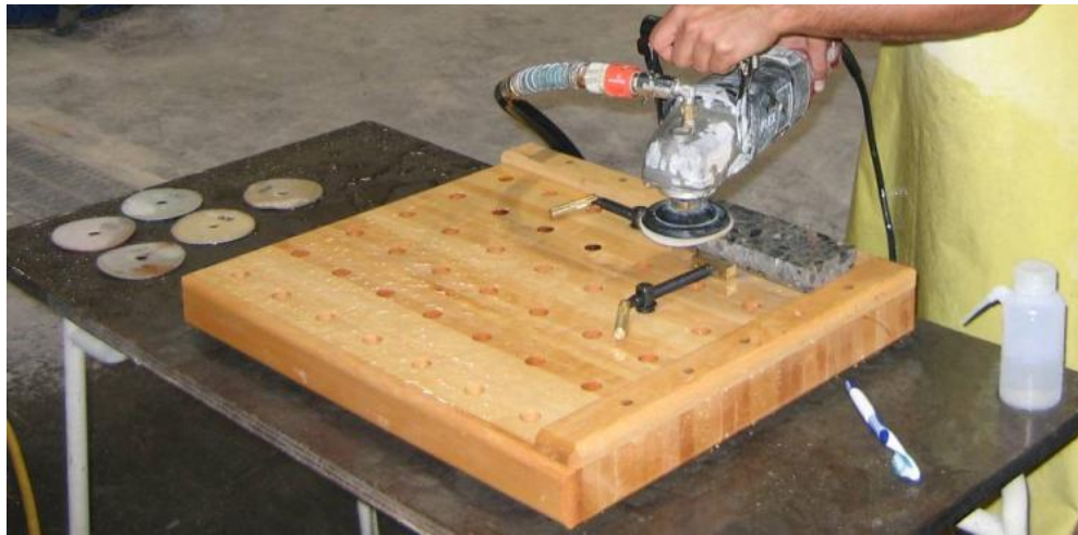
Figure 1: Polishing process of the concrete specimens for the Gel Pat Test.
