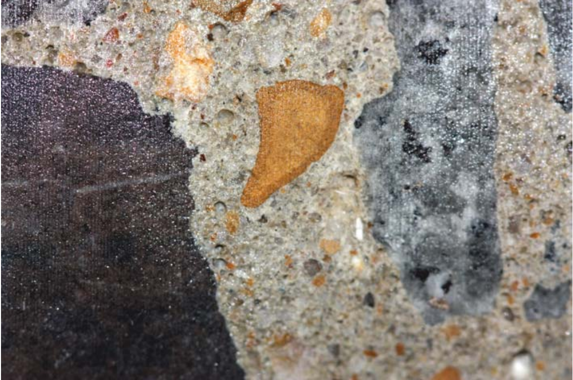
Figure A2: Details on the core Ark-1; reaction rim on a reactive particle of the fine aggregate.
