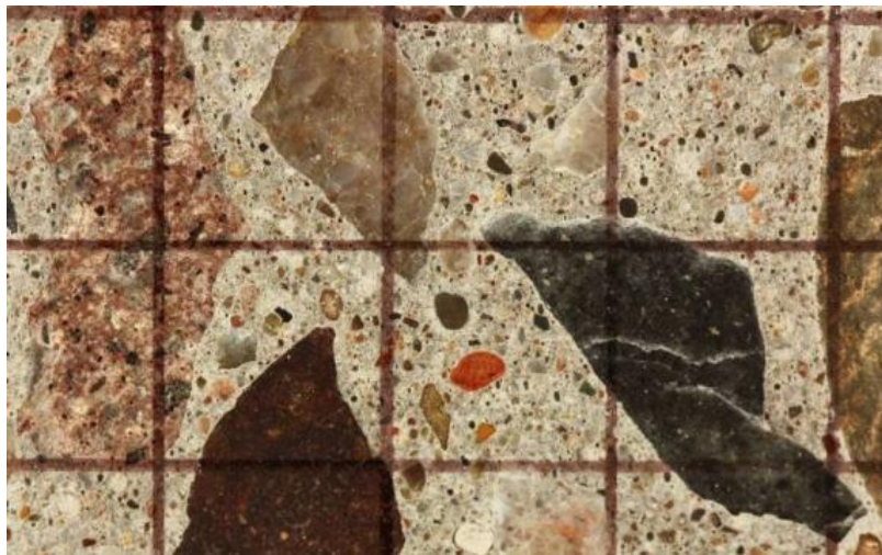
Figure 2: One cm by one cm (0.4 in. by 0.4 in.) grid drawn at the surface of the polished concrete section for petrographic examination using the DRI method.
