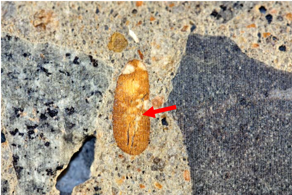
Figure A6: Details on core Ark-3. A: reaction rim around reacted sand particle and air void filled with alkali-silica reaction product; B: cracks with alkali-silica reaction product in a reactive particle of the fine aggregate.
