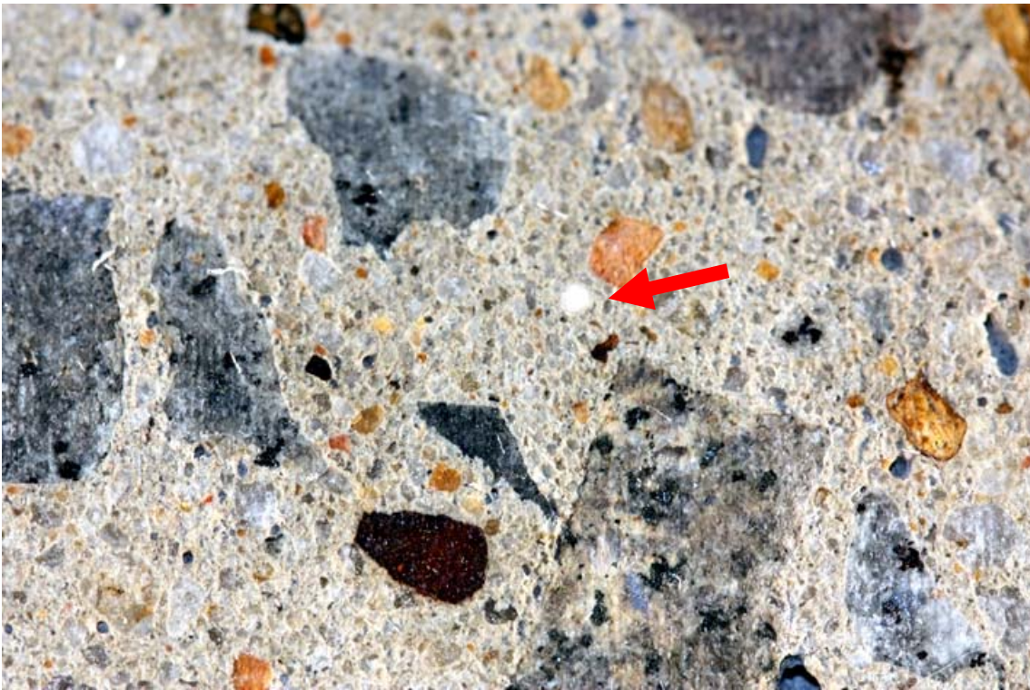
Figure A10: Details on core Ark-5. A: reaction rim and cracks with alkali-silica reaction product in a reacted particle of the fine aggregate; B: air void filled with alkali-silica reaction product.
