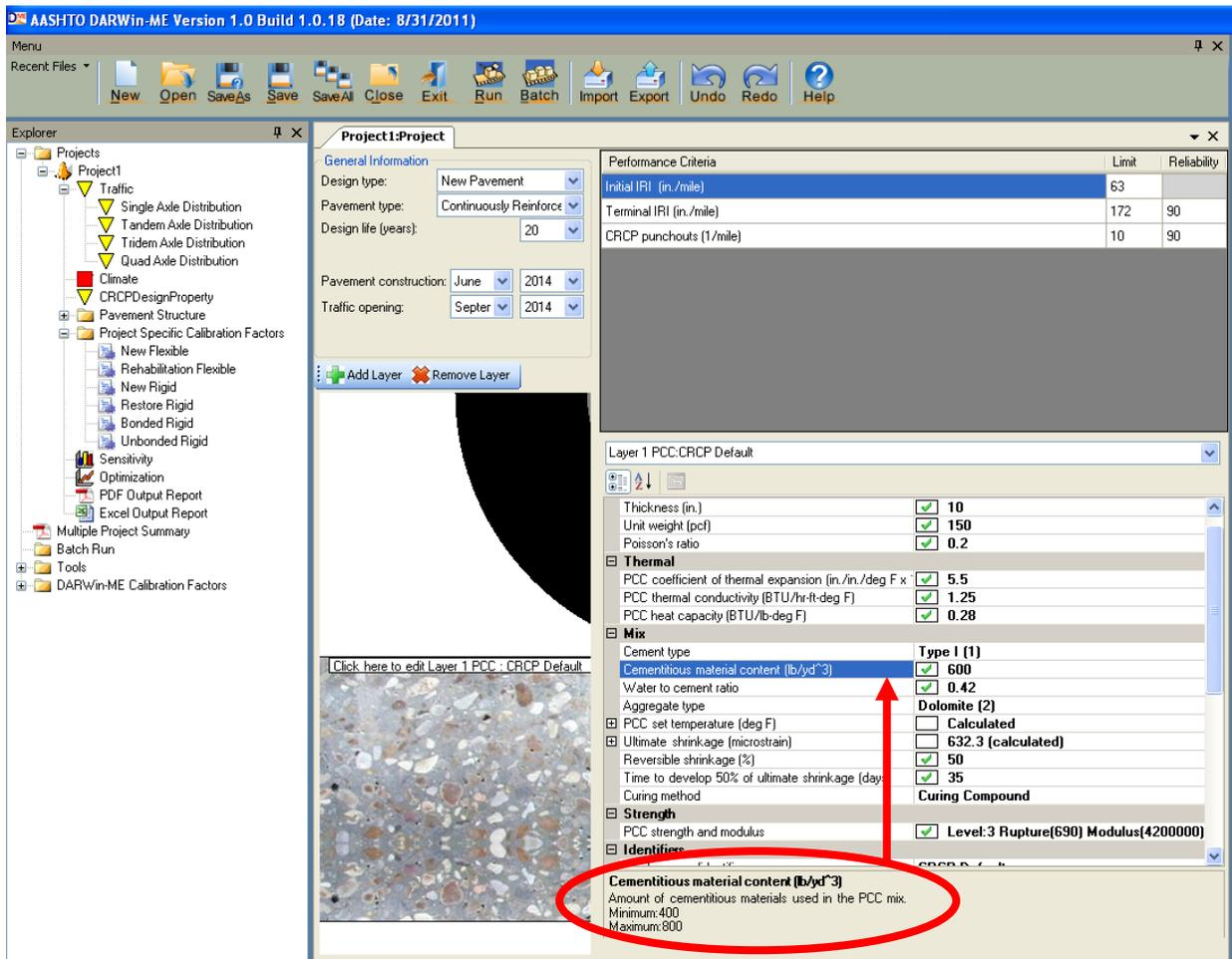
Figure 3. Pavement type selection, CRCP performance criteria, and PCC material properties in the AASHTO Pavement ME Design program.
