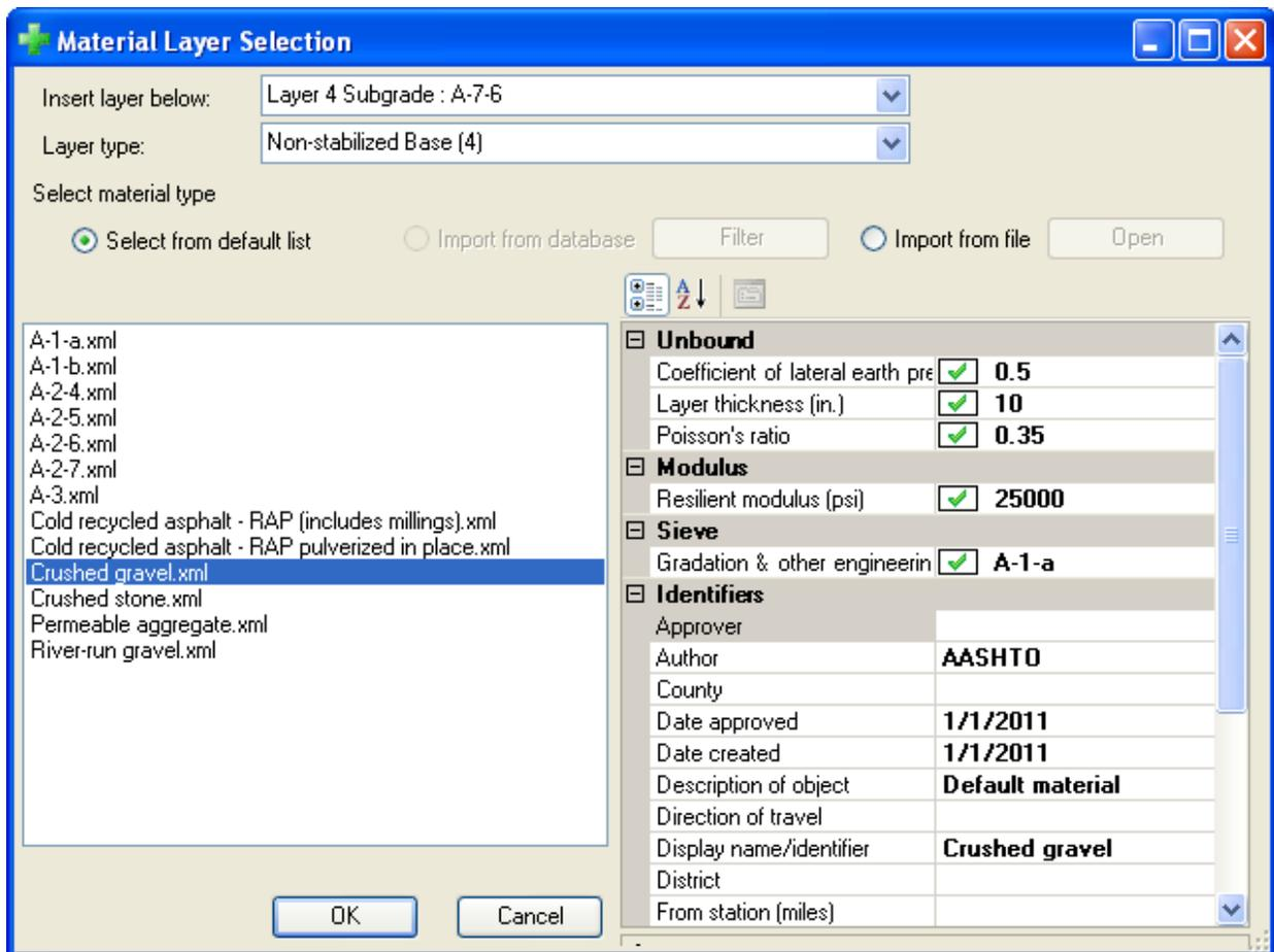
Figure 4. Selecting support layer types and properties in AASHTO Pavement ME Design.
