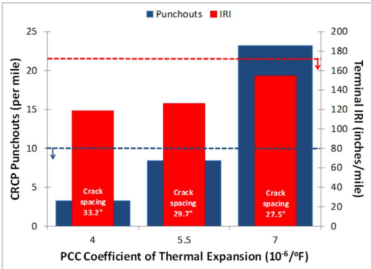
**Figure 14. Impact of PCC CTE on predicted CRCP punchouts and terminal IRI.**
