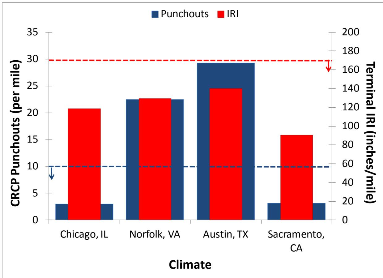
**Figure 18. Impact of climate on predicted CRCP punchouts and terminal IRI.**
