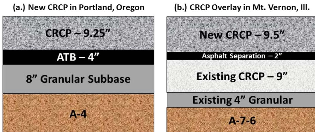
**Figure 19. Example design cross sections for (a) new CRCP in Portland, OR, and (b) CRCP overlay near Mount Vernon, IL.**
