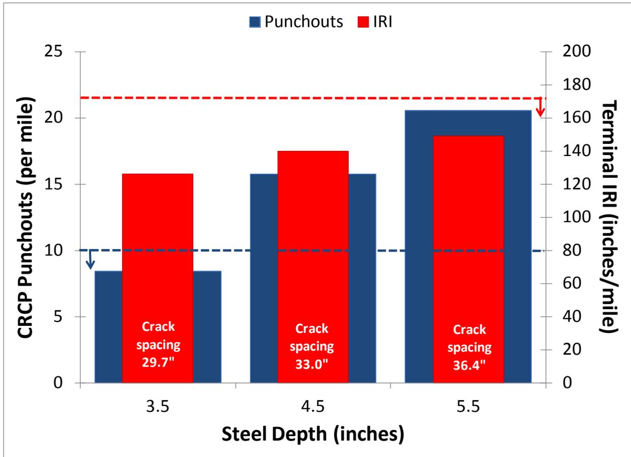
**Figure 13. Impact of depth of reinforcing steel at 0.7 percent on predicted CRCP punchouts and terminal IRI.**
