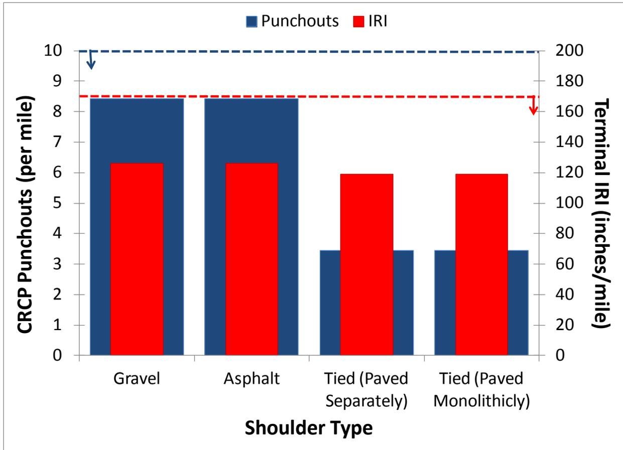
**Figure 15. Impact of shoulder type on predicted CRCP punchouts and terminal IRI.**
