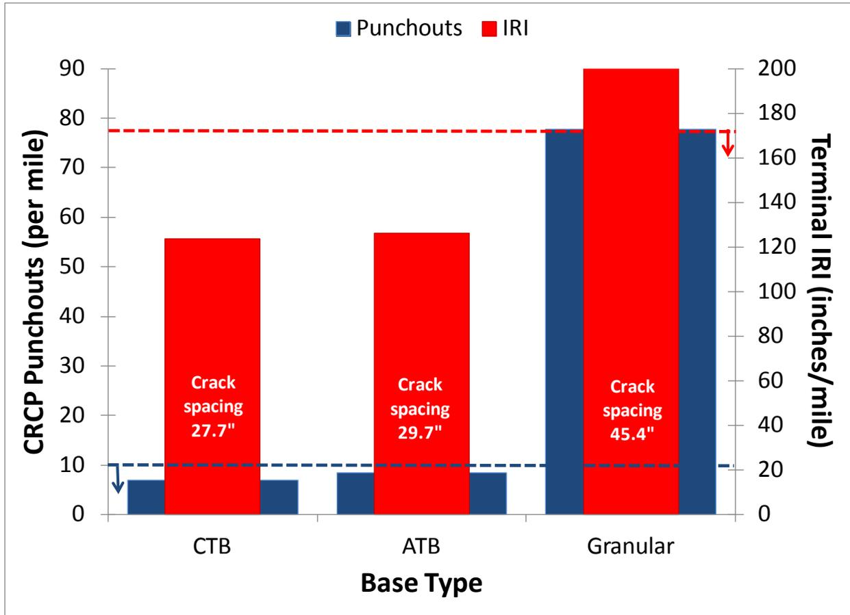
**Figure 16. Impact of base type and associated friction on predicted CRCP punchouts and terminal IRI.**
