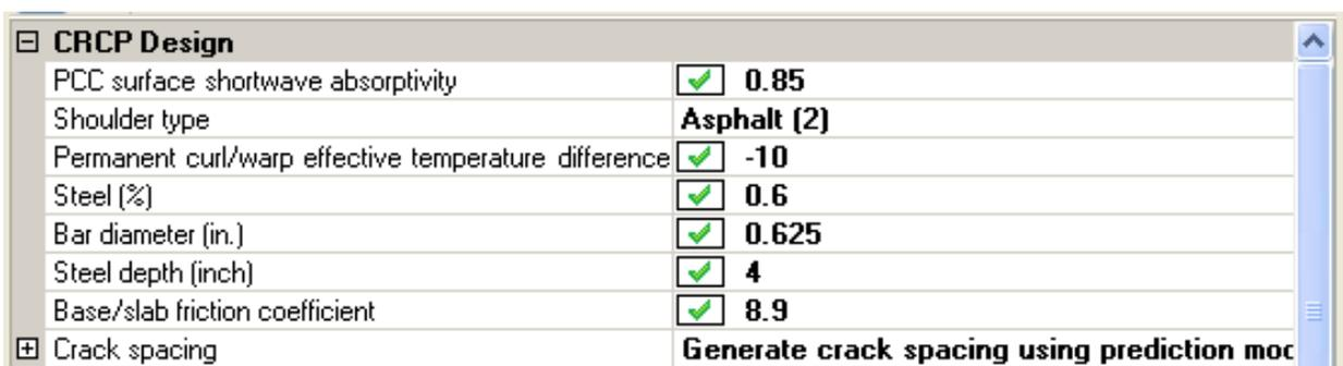
Figure 5. Input menu for CRCP reinforcement properties, base/slab friction, permanent curl, shoulder type, and short-wave absorptivity.
