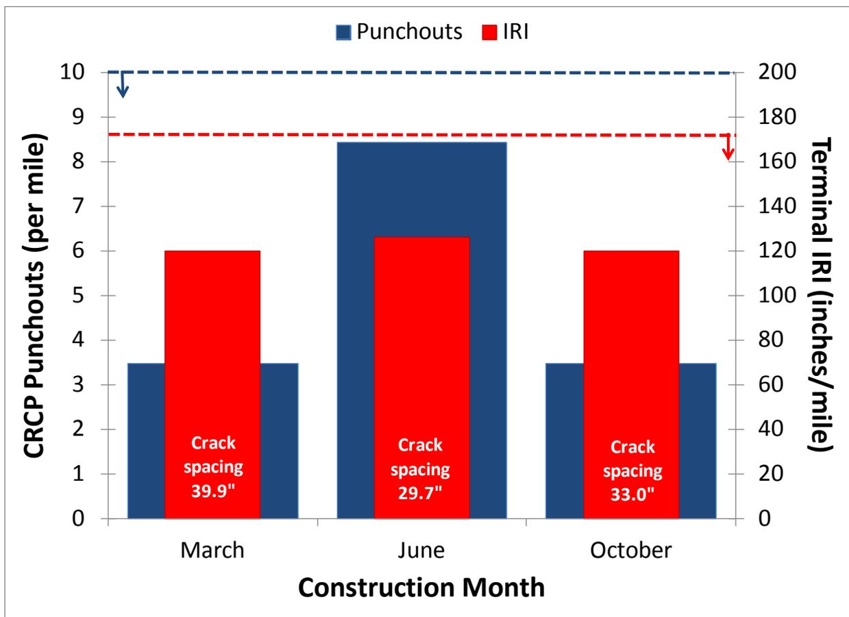
**Figure 17. Impact of construction month on predicted CRCP punchouts and terminal IRI.**
