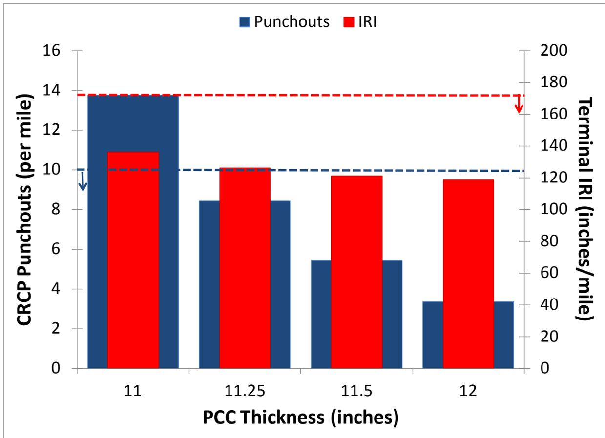
**Figure 11. Impact of PCC thickness changes on predicted CRCP punchouts and terminal IRI.**
