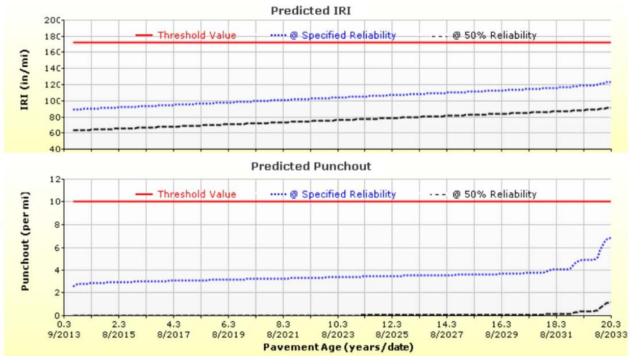
**Figure 10. Example of IRI and punchout predictions for 50-percent and specified reliability over time.**
