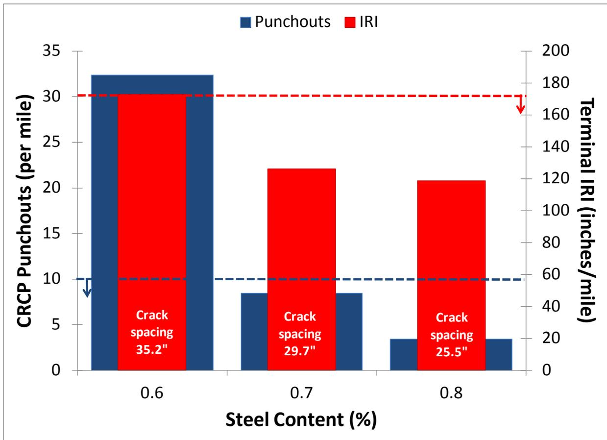
Figure 12. Impact of reinforcing steel percentage on predicted CRCP punchouts and terminal IRI.
