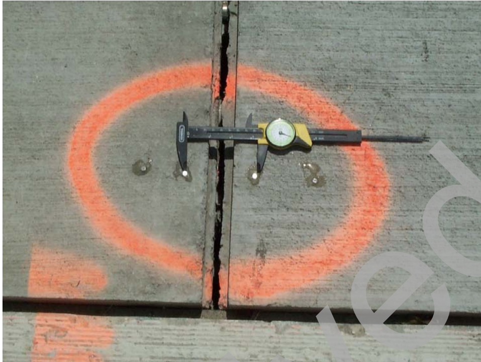
Figure 41. Photo. Dial calipers were used to measure expansion joint movement using Demec points on either side of the joint as gage points.
