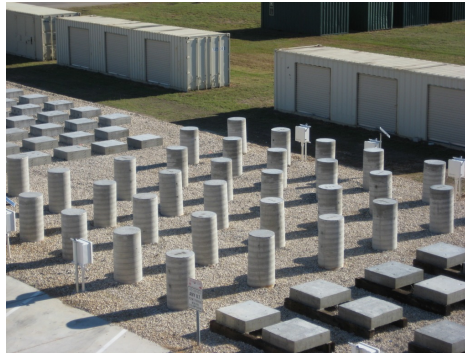
Outdoor Field Site at the University of Texas at Austin. A total of 64 "bridge deck", 36 "column", and 60 "slab" specimens were cast for research under this program.
