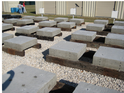
Close-up of bridge decks cast at the Concrete Durability Center at the University of Texas at Austin.
