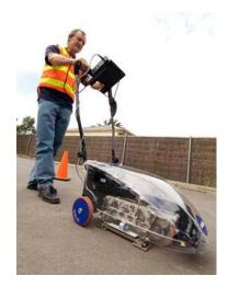
Figure 14. SSI CS8800 (www.smoothroad.com) walking profiler.
