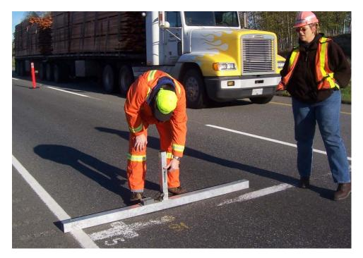
Figure C-1. Rut depth survey (BCMoTI 2012).
