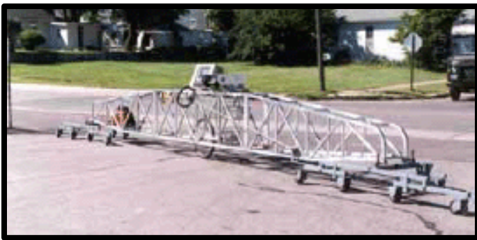
Figure 1. Truss-type California profilograph. (Perera, Kohn, and Tayabji 2005)
