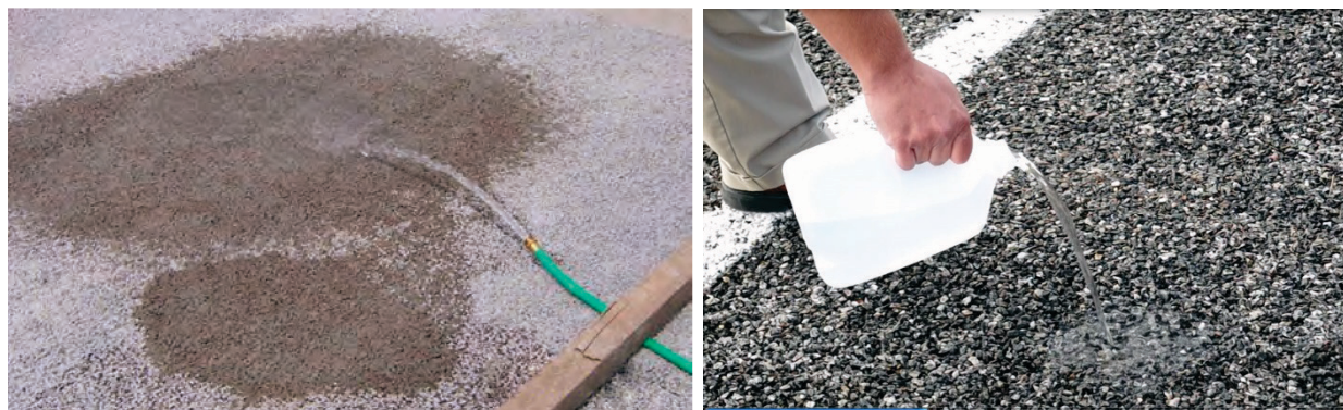
Figure 6-13. Pervious concrete (left, courtesy John Kevern) and porous asphalt (right, courtesy National Asphalt Pavement Association).
