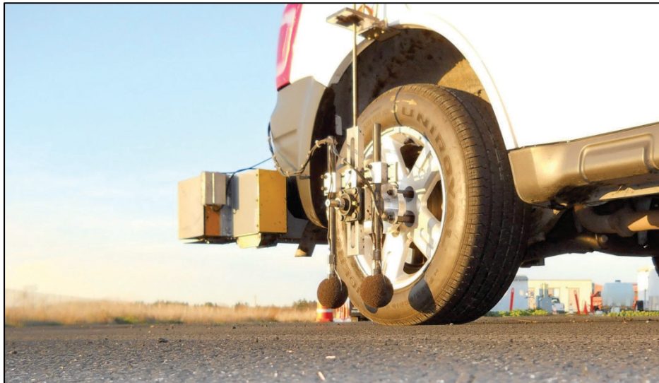
Figure 6-6. On-Board Sound Intensity (OBSI) setup (photo courtesy of John Harvey).
