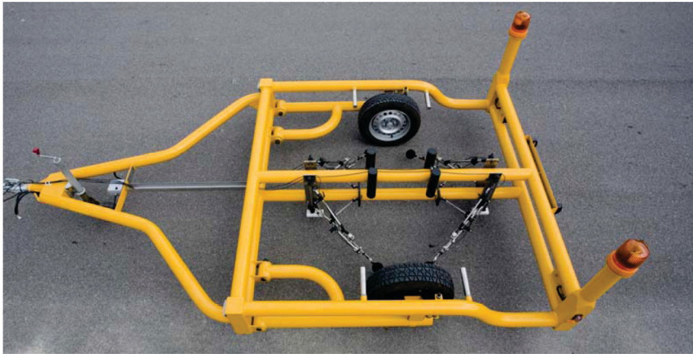
Figure 6-5. Close Proximity (CPX) test trailer (Bendtsen and Thomsen 2008).
