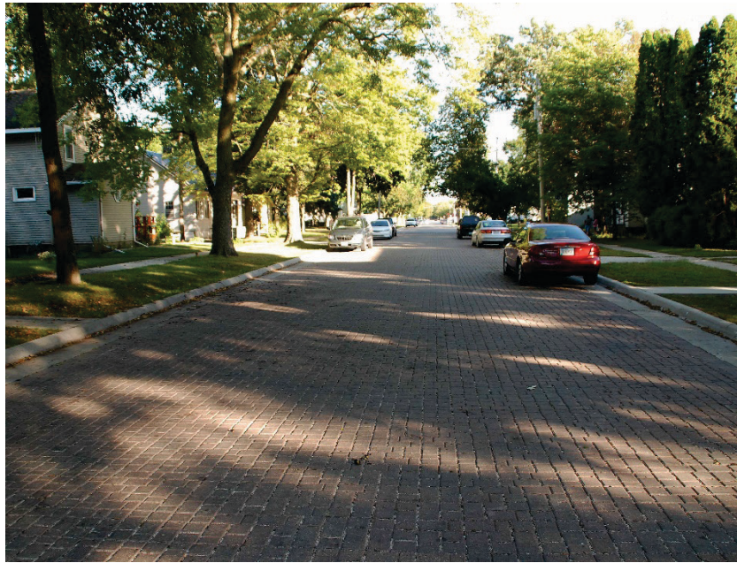
Figure 6-14. Permeable interlocking concrete pavers (courtesy Interlocking Concrete Pavement Institute).
