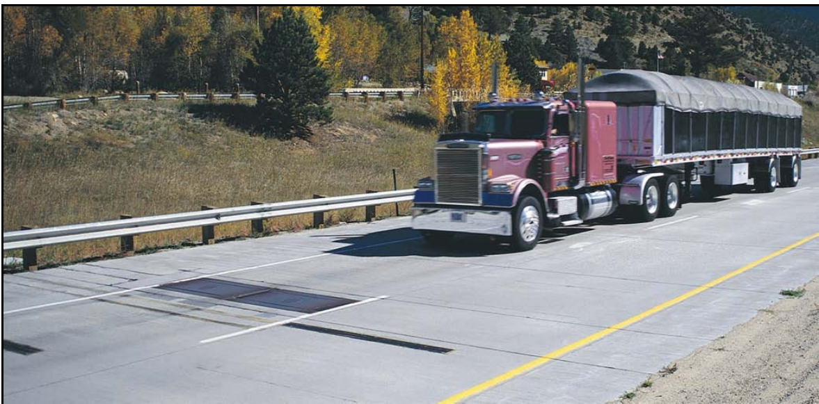
Figure 3. Photo. In-line weigh sensors (single load cells), a trailing axle sensor, and detection loops (single threshold system).
