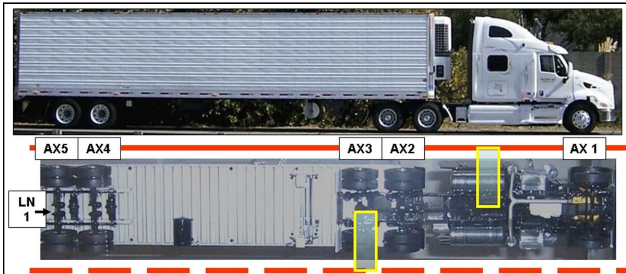
Figure 55. Photo. Class 9, Type 3S2 typical axle and wheel alignment crossing right and left weigh sensors.
