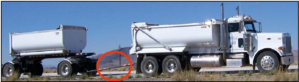
Figure 38. Photo. Class 9 Type 32 with long towbar.
