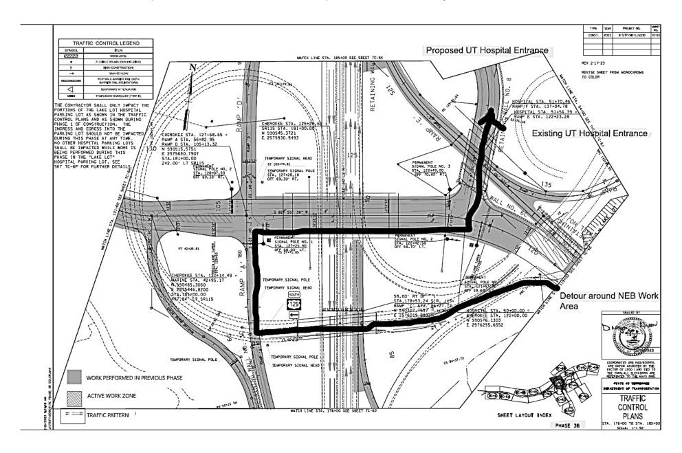
This sheet depicts the traffic pattern in the interchange in Phase 3C. The work in the hatched area in Phase 3B has been completed and traffic on Cherokee Trail now has access to the new UT Hospital Entrance without having to cross over SR-115, Alcoa Highway.
