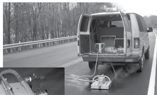
Top: The Dynamic Friction Tester in use in Maryland.
