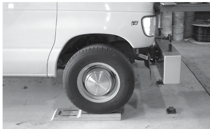
The height sensors of an inertial profiler are checked. Such profilers can be used to obtain pavement smoothness data.
