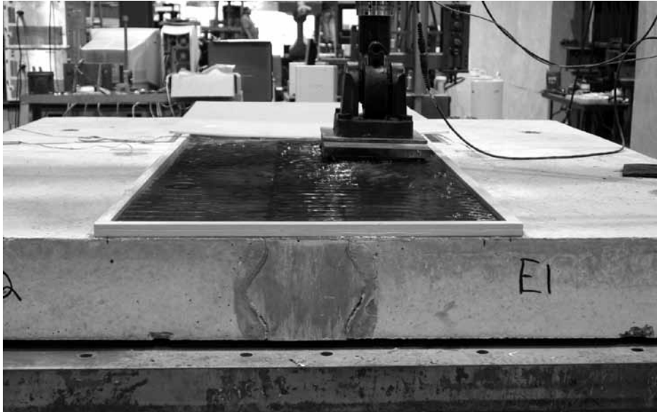
Ultra-high performance concrete connections are tested at FHWA's Turner-Fairbank Highway Research Center in McLean, VA. These connections can link prefabricated bridge girders to precast concrete bridge decks.
