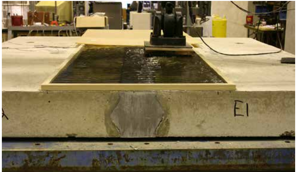
Ultra-high performance concrete (UHPC) can improve the connections used to link bridge girders to precast concrete bridge decks. Here, UHPC connections are tested at FHWA's Turner-Fairbank Highway Research Center in McLean, VA.
