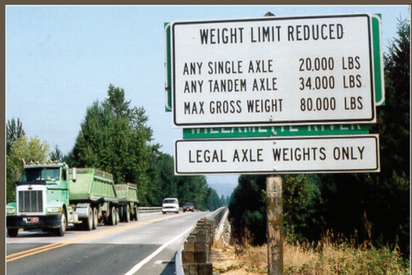
Figure 12. State agencies reduce weight limits on certain bridges for safety and to prevent further deterioration. Source: Bala Sivakumar, HNTB Corporation.
