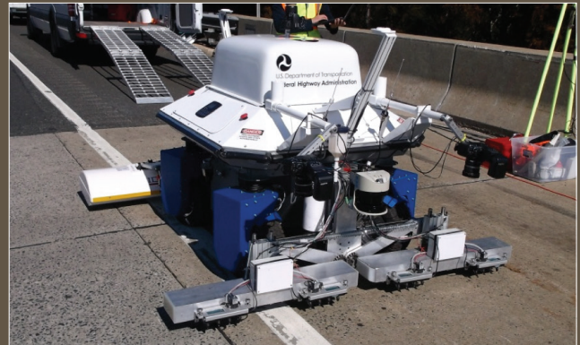
Figure 5. LTBP RABIT™ bridge inspection tool at the NJ Rt. 55 over Porchtown Road steel multigirder cluster bridge.
