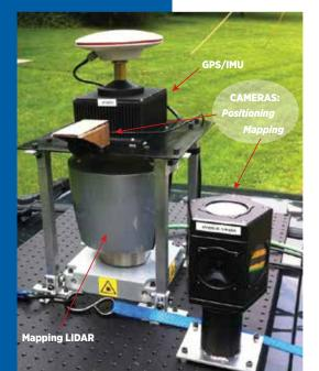
Feature-based mapping and positioning sensor suite showing a GPS/IMU (inertial measurement unit) box and a forward-looking camera for positioning, and a 360-degree camera and Velodyne<sup>®</sup> LIDAR for mapping.
