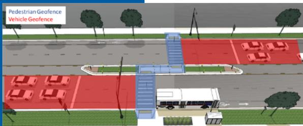
Transportation researchers are exploring methods of implementing MANETs to enhance communication between vehicles and nonmotorized travelers. © University of Virginia.
