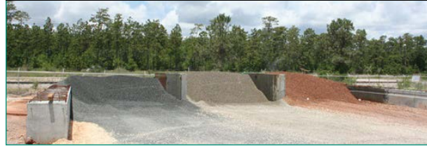
Figure 1. Lightweight aggregate stockpiles with continuous sprinklers.
