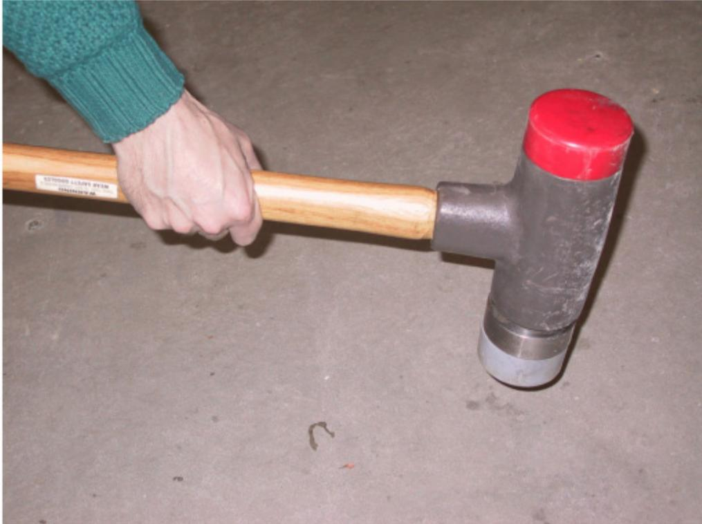
Figure 17. Photo. Twelve-pound impulse sledge hammer with soft gray rubber tip.
