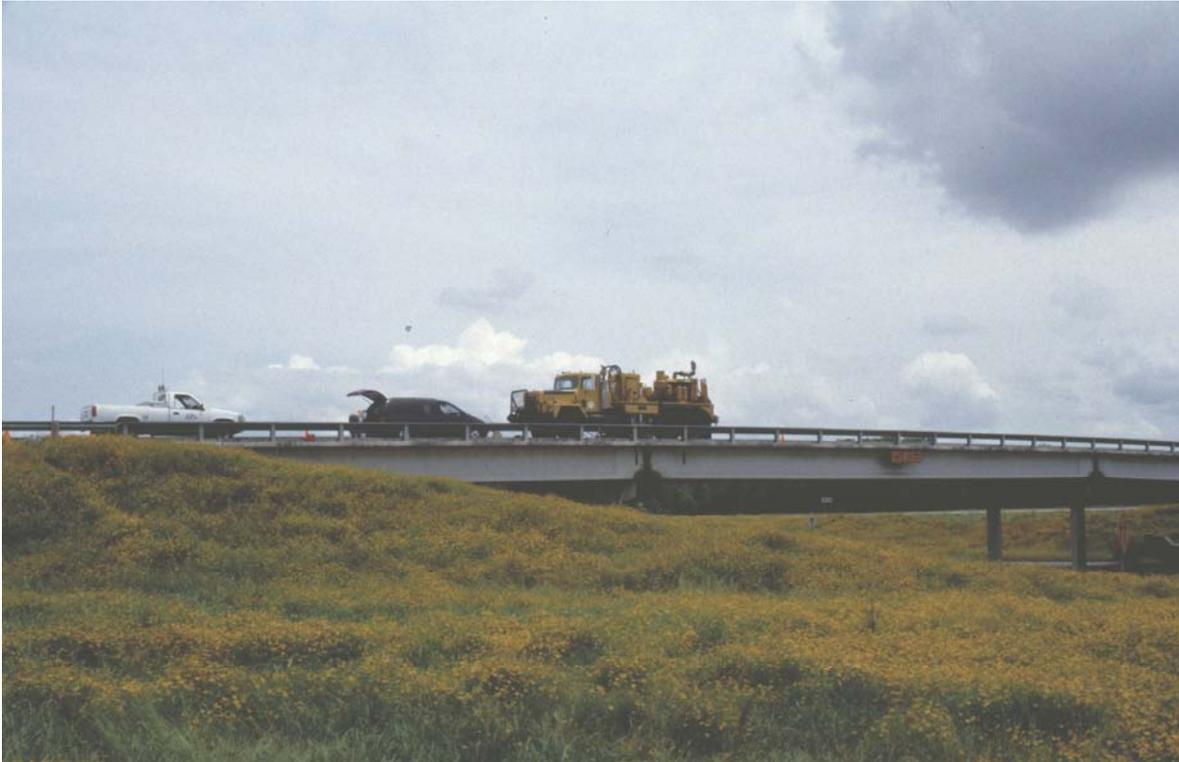
Figure 9. Photo. Vibroseis truck over the east pier, Old Reliance Bridge.
