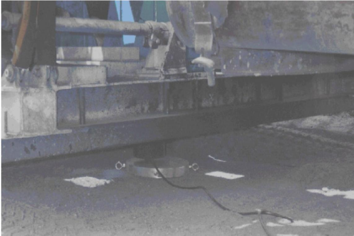
Figure 21. Photo. Vibroseis single-point-plate loading system.
