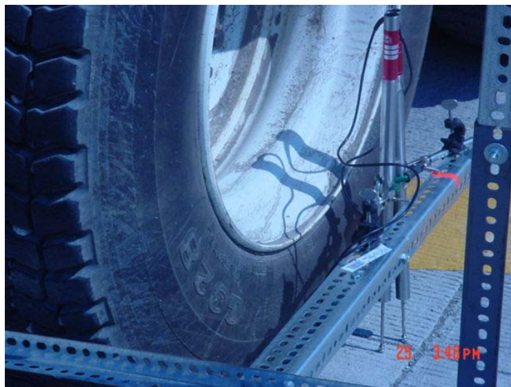
Figure 78. Photo. Two LVDTs measuring pavement deflections across a joint.
