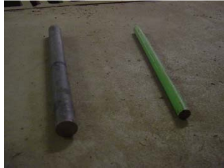
Figure 4. Photo. Steel dowels 3.81 and 2.54 cm (1.5 and 1.0 inches) in diameter.
