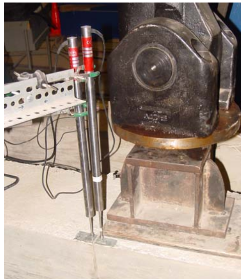
Figure 17. Photo. LVDTs positioned on both sides of the joint.
