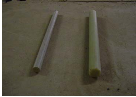
Figure 3. Photo. FRP dowels (2.54 and 3.81 cm (1.0 and 1.5 inches) in diameter).
