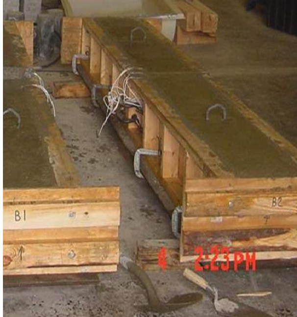
Figure 12. Photo. Surface finished specimens.
