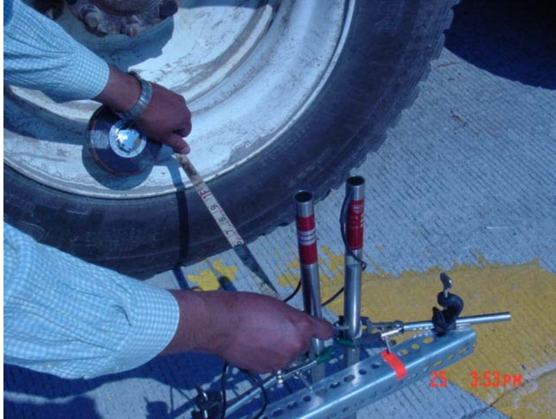
Figure 79. Photo. Measuring distance from tire to LVDTs (when loading is away from the selected dowel).
