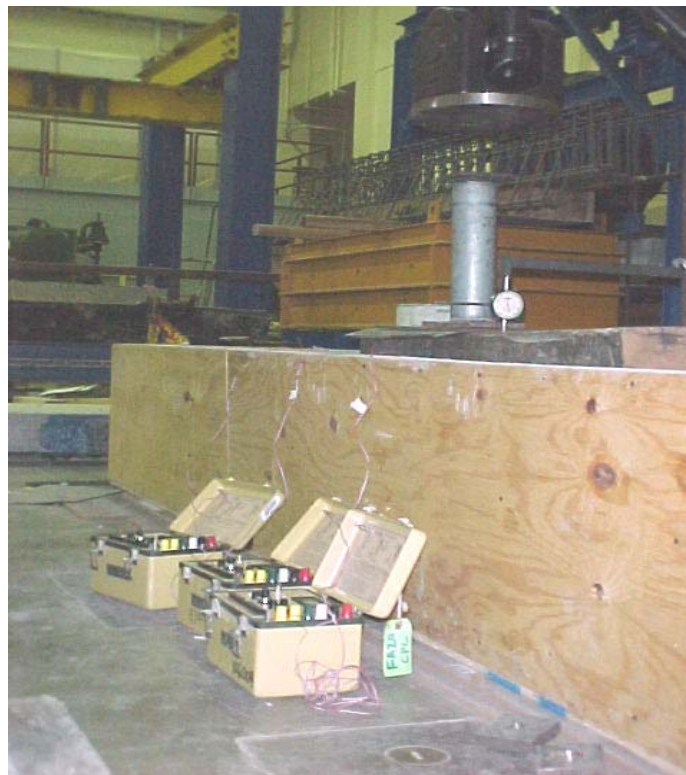
Figure 110. Photo. Lab test of timber tie with FRP dowel bar as the load transfer device.
