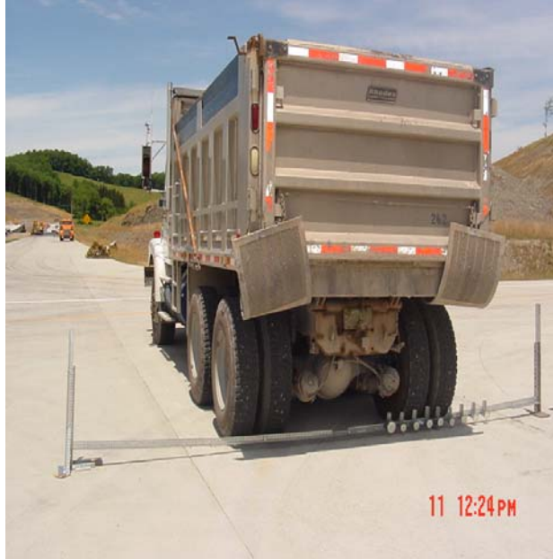
Figure 64. Photo. Dial gauges for measuring pavement deflection under truck loading.
