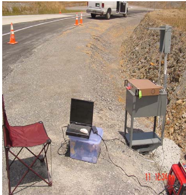
Figure 65. Photo. Data acquisition system used for field tests.
