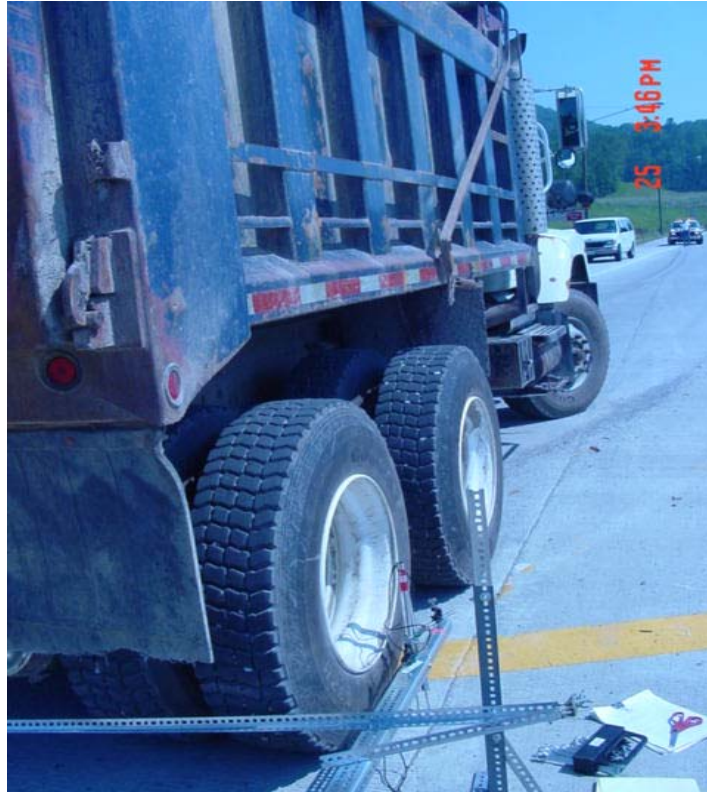
Figure 77. Photo. WVDOT truck positioned near a joint for the test.
