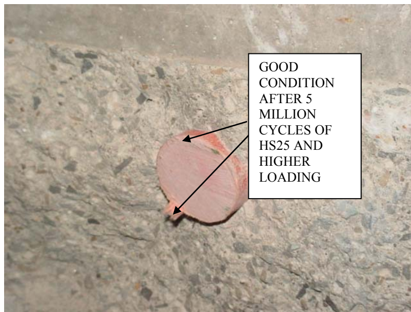
Figure 44. Photo. Dowel-concrete interface condition in slab number 4 after 5 million load cycles.
