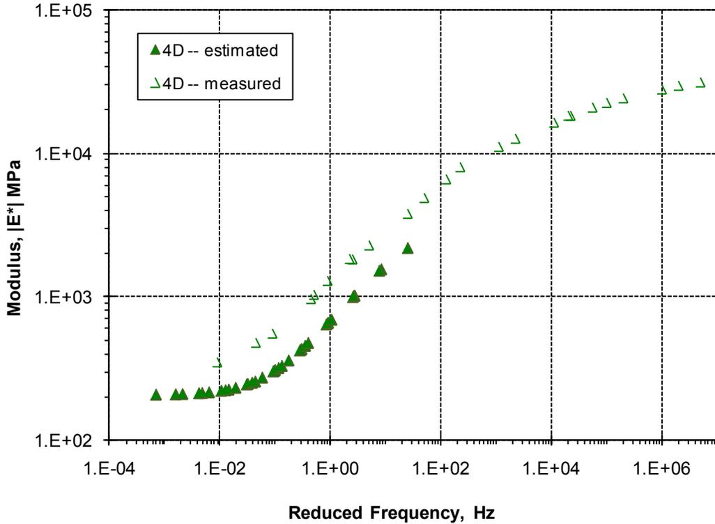
**Figure 21. Graph. Example of poor blending (mix 4D).**
