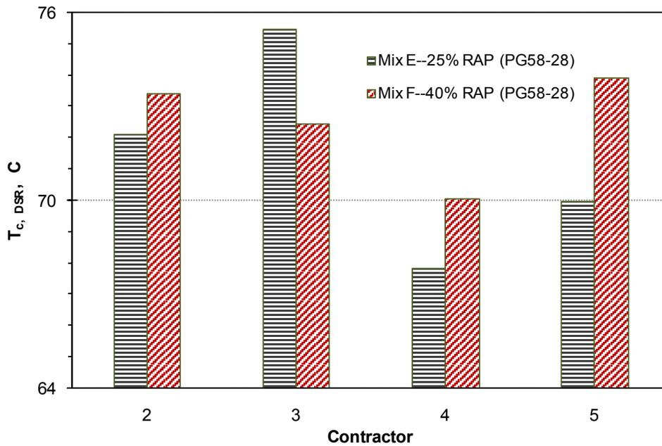
**Figure 46. Graph. DSR critical temperatures—mixes with PG58-28 binder.**
