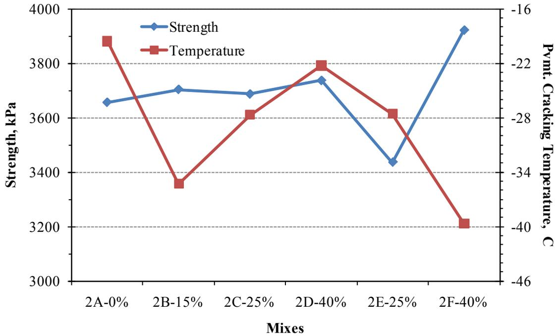
Figure 25. Graph. IDT strength and pavement cracking temperature for contractor 2.
