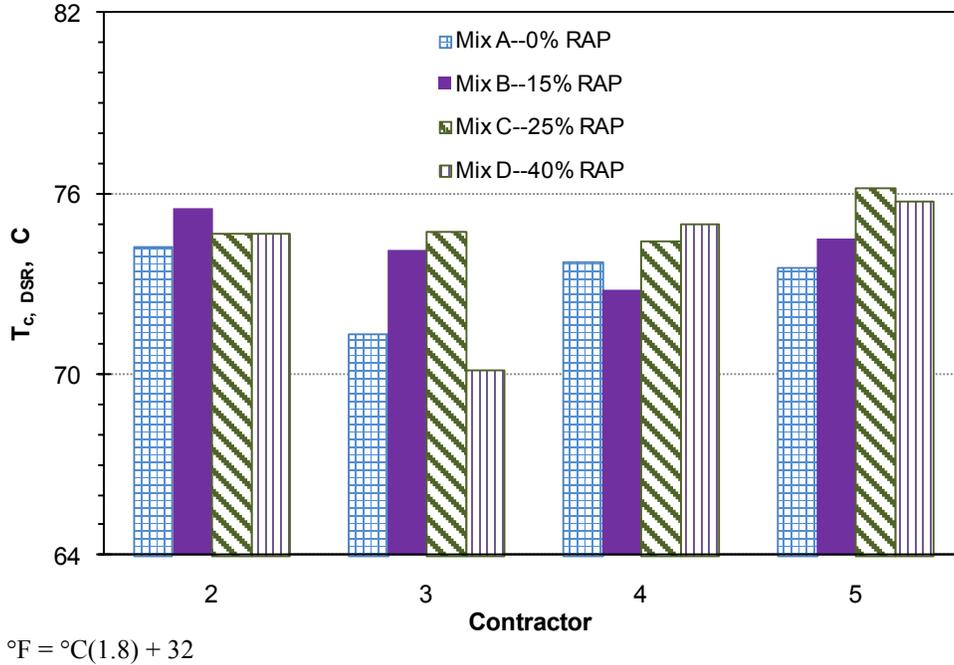
**Figure 45. Graph. DSR critical temperatures—mixes with PG64-22 binder.**
