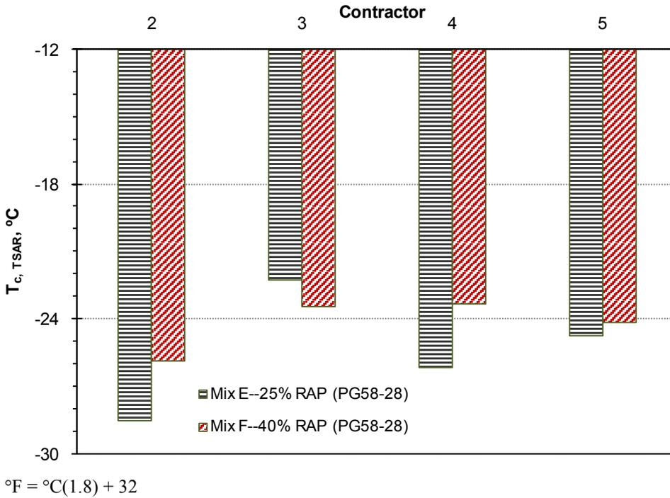
Figure 52. Graph. TSAR™ critical temperature—mixes with PG58-28 binder.
