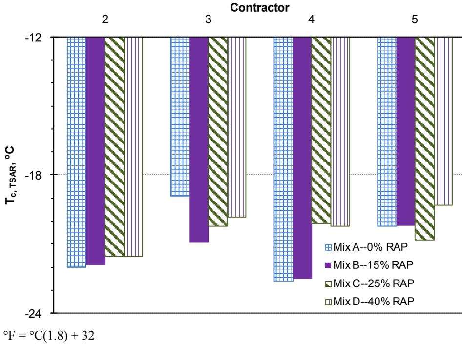
Figure 51. Graph. TSAR™ critical temperature—mixes with PG64-22 binder.
