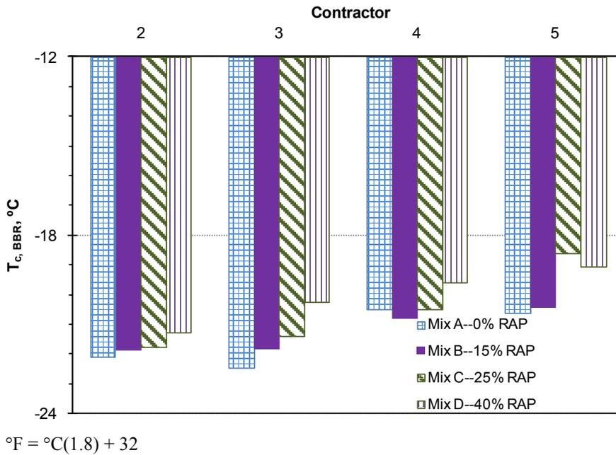
**Figure 48. Graph. BBR critical temperatures—mixes with PG64-22 binder.**
