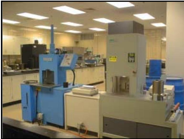
**FIGURE 1 Pine and Troxler Superpave gyratory compactors.**
