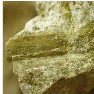
**Figure 3. Photograph of the lithium-bearing mineral spodumene.**
