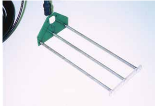
FIGURE 7.4. The moisture probe designed at the FHWA highway research center.
