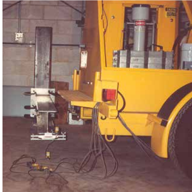
FIGURE 6.8. An FWD being calibrated at the PennDOT regional calibration center early in the LTPP program.
