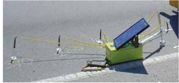
FIGURE C.5. Automated Temperature Datalogger setup in the field. The Datalogger is powered by a 12-volt SLA battery. The solar panel charges the battery to sustain 12 volts during data collection.
