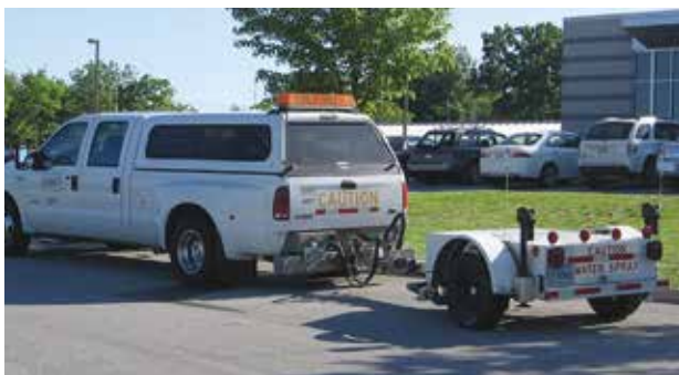
FIGURE 6.16. Locked-wheel skid tester currently in use for collecting friction data.
