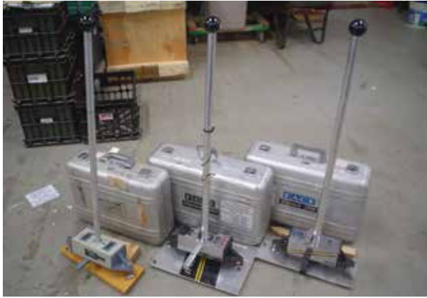
FIGURE 6.28. Three Face® Dipstick® profile measuring devices with carrying cases. Left to right are the 1500, 2000, and 2200 models.
