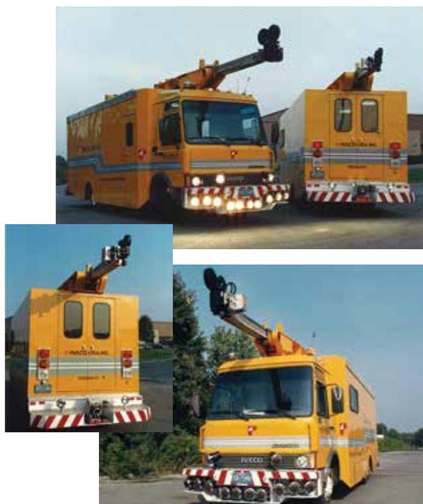
FIGURE 6.9. Mobile equipment used to photograph pavement distress. Mounted on a boom extending from the front of the vehicle is the motion picture camera, synchronized with vehicle speed for continuous filming; flood lights are mounted on the custom front bumper. On a boom extending from the rear of the vehicle is a 35-mm pulse camera, which collects transverse profile. The camera is controlled by a distance measuring instrument that can trigger the camera at preset intervals; a strobe projector is mounted on the rear bumper.
