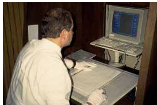
FIGURE 6.26. Translating photographs produced by the automatic profilers into digital format. Transverse profile/rutting was determined from 35-mm picture frames by the string line method/algorithm. Generally 30 points defined the transverse profile.
