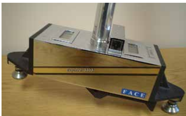
FIGURE 6.21. Manual Face® Dipstick® used to collect profile data in the LTPP program.
