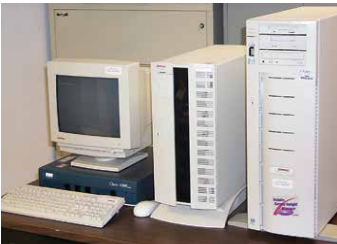
FIGURE 8.7. The LTPP DEC Alpha 3000 AXP 400 S computer system running the UNIX® operating system, used for NIMS server functions from 1993 to 1997.
