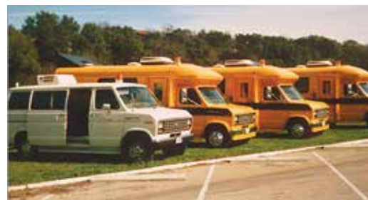
FIGURE 6.17. The first (DNC 690) Profilometers used in the LTPP program. Three were mounted in the Champion motor home chassis with Ford underpinning with dual rear wheels, and the fourth in a Ford E350 van chassis.
