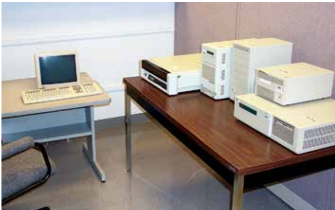
FIGURE 8.7. The LTPP DEC Alpha 3000 AXP 400 S computer system running the UNIX® operating system, used for NIMS server functions from 1993 to 1997.
