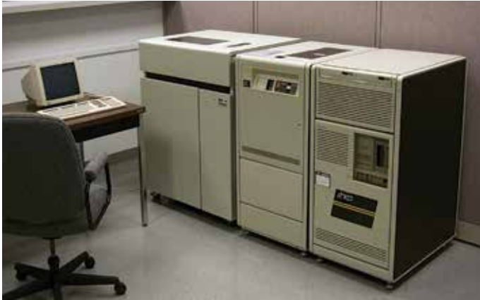
FIGURE 8.6. DEC MicroVAX 3900 computer running the UNIX® operating system, used as the first LTPP National Information Management System (NIMS) server from 1989 to 1993.
