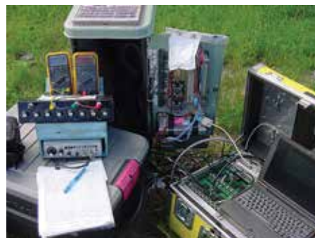
FIGURE 7.3. Mobile monitoring equipment for downloading data collected at seasonal monitoring sites.
