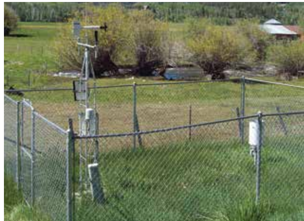
FIGURE 6.2. Complete automated weather station installation with protective fencing.
