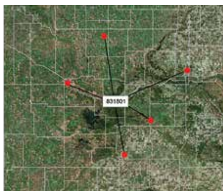
FIGURE 6.4. A virtual weather station (VWS). This example shows the locations of five operating weather stations used to create the VWS for GPS section 831801 on Trans-Canada Highway 1 in southwestern Manitoba.
