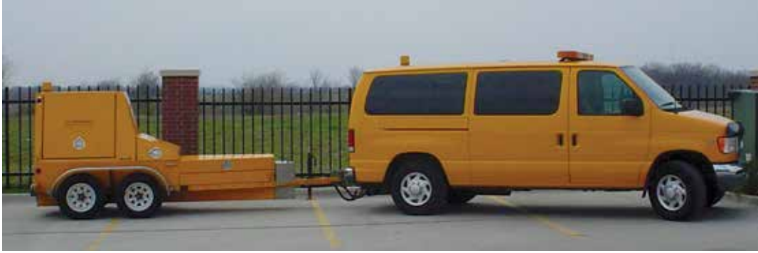
FIGURE C.3. One of the four original FWD van and trailer units.
