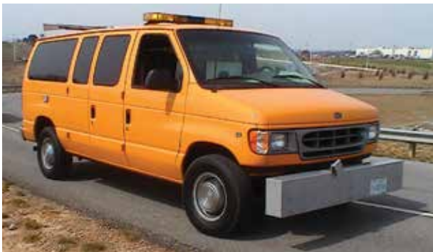
FIGURE 6.19. ICC profiler MDR 4086L3 (Ford E350 van), in use from 2002 to 2013.
