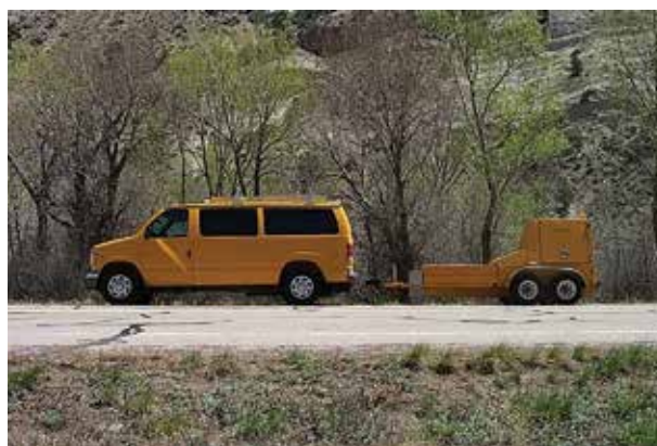
FIGURE 6.5. Van-towed falling weight deflectometer equipment used in the LTPP program.
