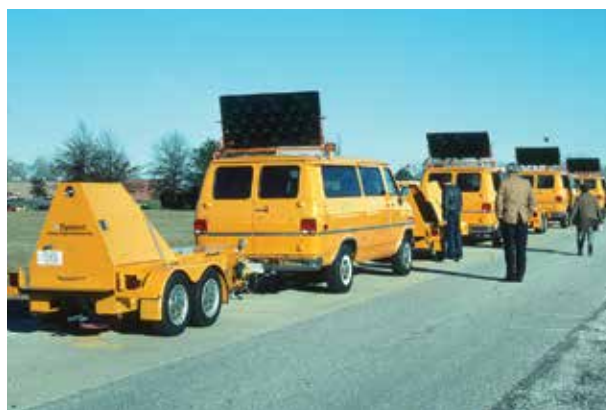
FIGURE 6.6. Falling weight deflectometer equipment at the first LTPP “thump-off,” which was held at Purdue University in November 1988.
