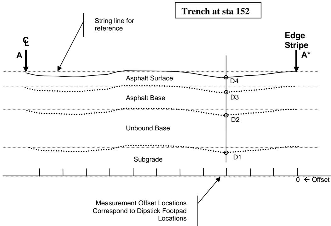
Distances (e.g. D1) are measured from the string line to the top of the layer. Layer numbers should correspond to the IMS layer number unless field conditions deviate from information contained in the database. Regardless, careful documentation of the layer description and measurements shall be made.
