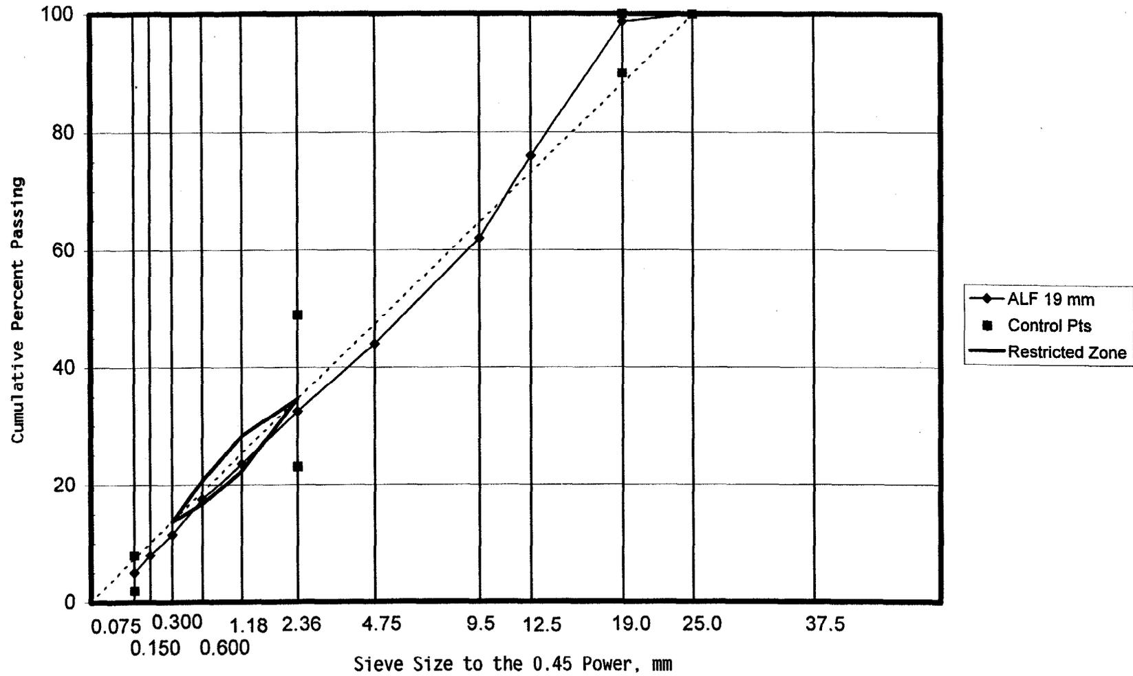
Figure 2. SM-3 aggregate gradation for the surface mixtures.
