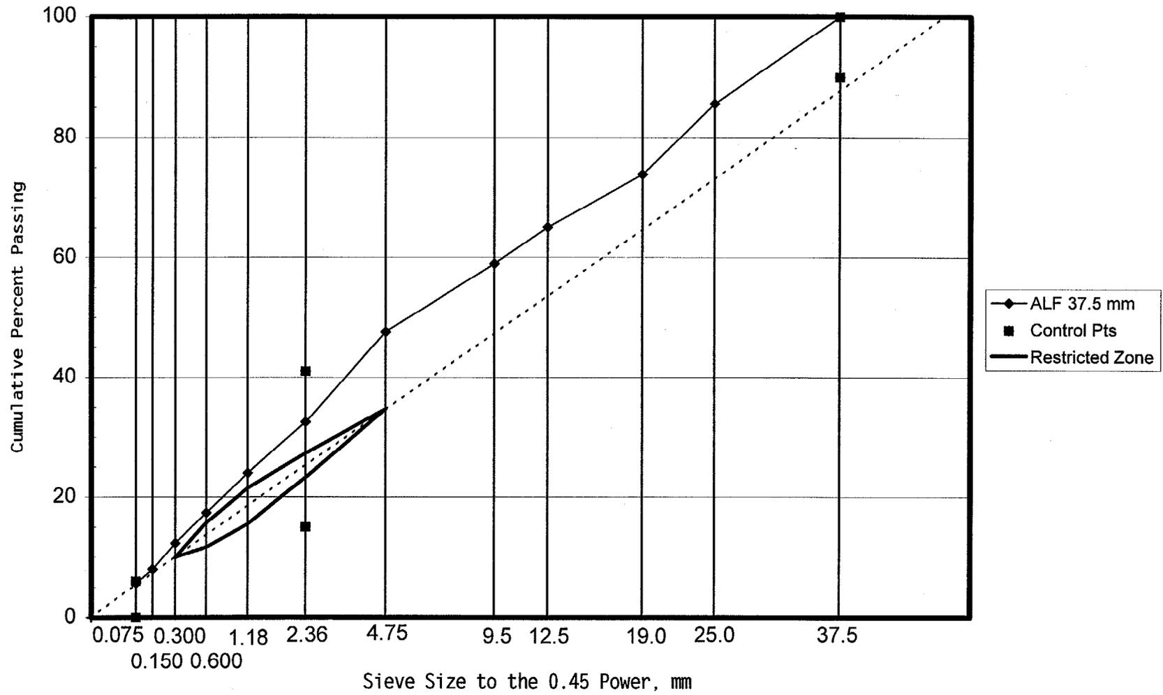
Figure 3. BM-3 aggregate gradation for the base mixtures.
