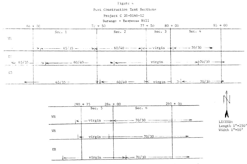
NOTE: In Figure 4 the data is referenced to the predominant mix in each test section. Cores were taken from the westbound driving lane of Sections 1-4.
