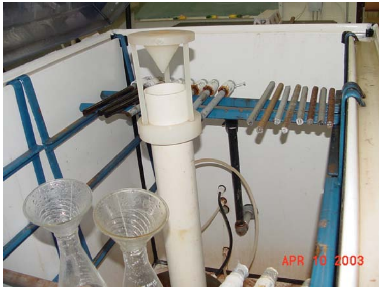
Figure 27. Bars positioned in salt fog chamber.
