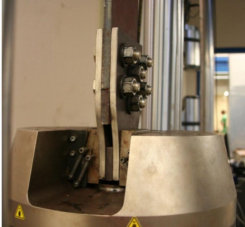
Figure 33. Photo. Frame 1 lower grip with specimen and grip adapter installed.
