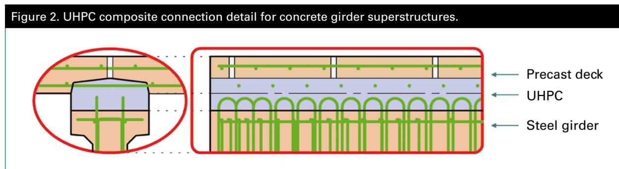
Figure 3. UHPC composite connection detail for steel girders.
