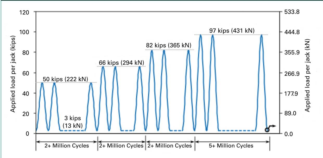
Figure 7. Horizontal shear fatigue ranges during cyclic testing.
