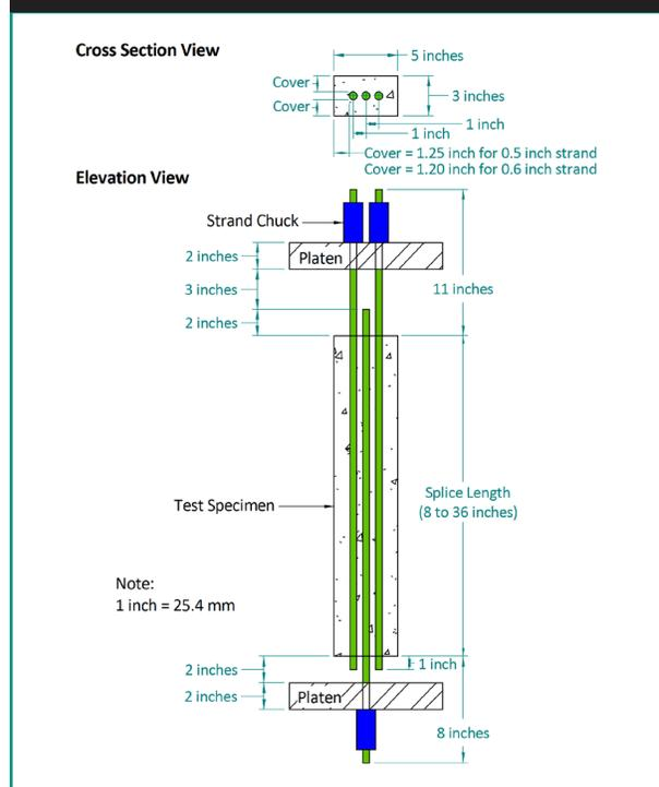
Figure 2. Casting of a 20-inch (50.8-cm) long test specimen.
