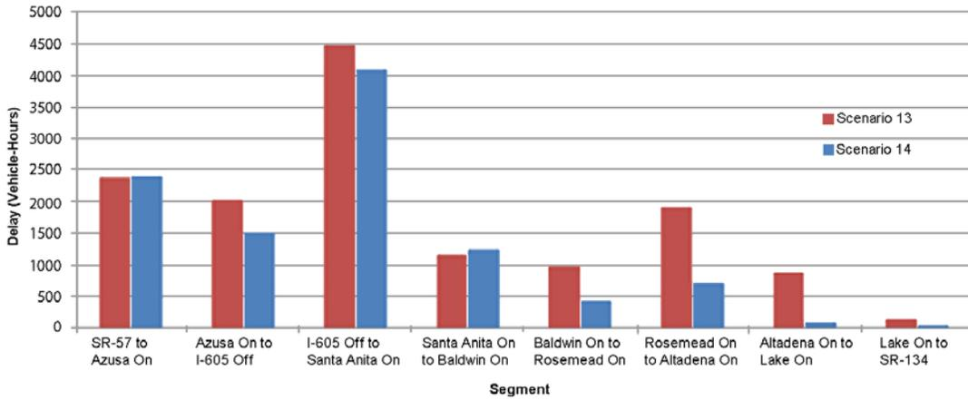
**Figure 29. Graph. Delay by segment for two scenarios in vehicle-hours—I-210 VISSIM simulation.**
