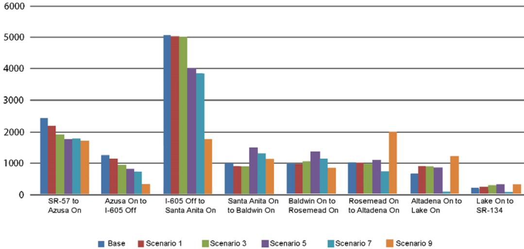
**Figure 30. Graph. Delay by segment for all scenarios in vehicle-hours—I-210 VISSIM simulation.**
