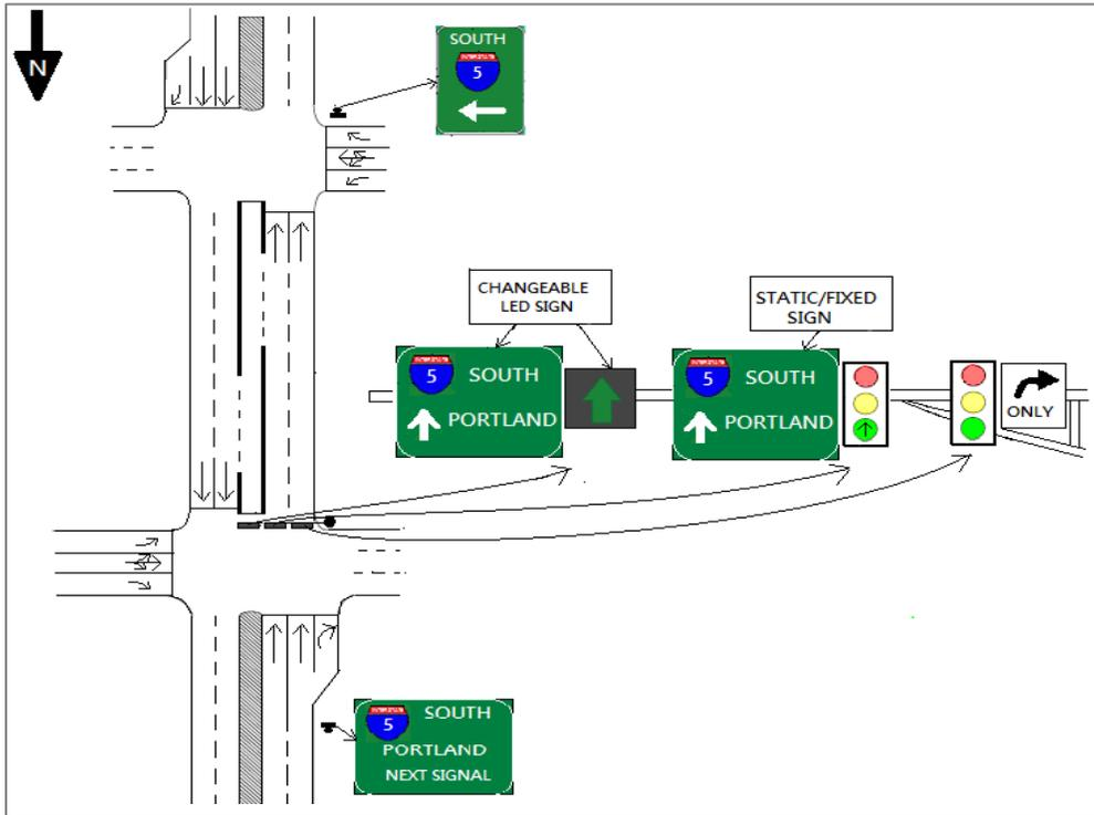
**Figure 86. Illustration. Proposed single-lane DRLT signalization during peak-period green phases.**
