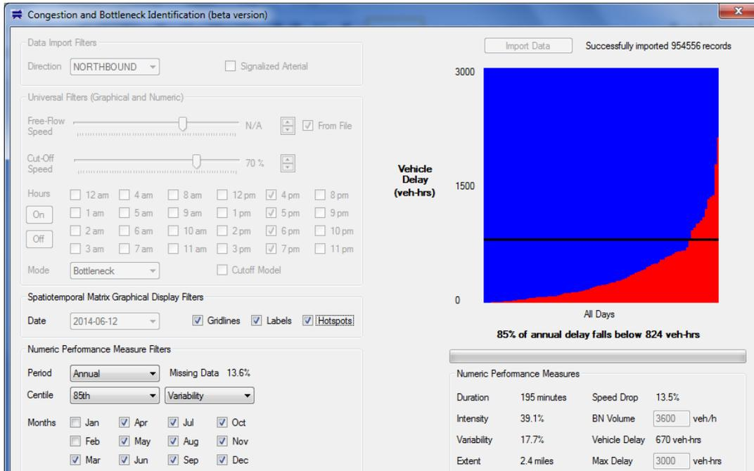
Figure 20. Screenshot. Newer CBI software tool featuring vehicle-hours of delay.
