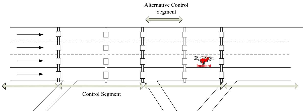
**Figure 76. Illustration. Dynamic HSR for incident response.**
