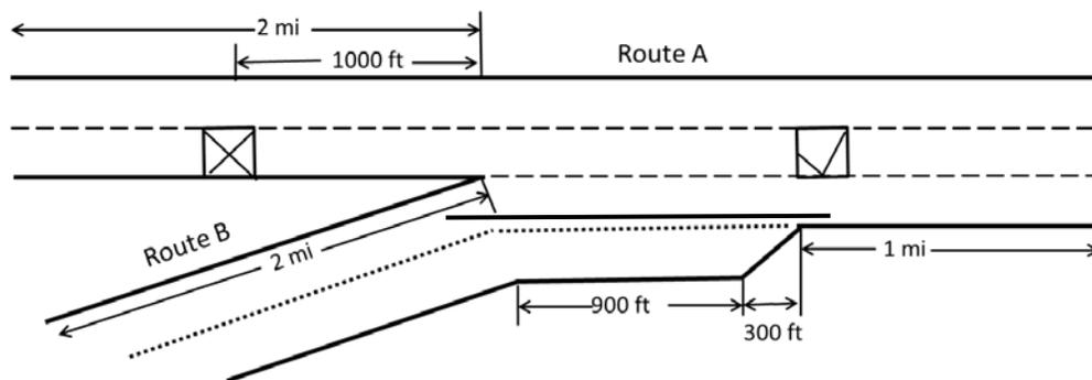
**Figure 50. Illustration. Merging of multiple two-lane freeways (closure on route A).**
