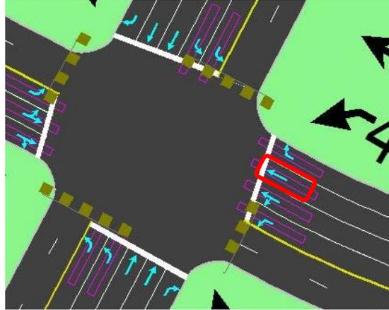
**Figure 41. Illustration. Lane assignment before DLG for case study 1.**
