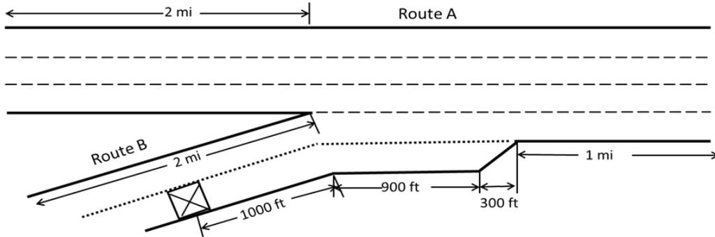
**Figure 51. Illustration. Merging of three- and two-lane freeways (closure on route B).**
