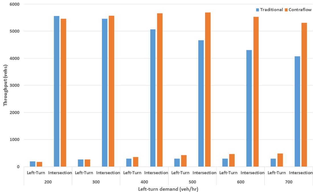
**Figure 97. Graph. Throughput increases due to CLT at various LT demand levels.**
