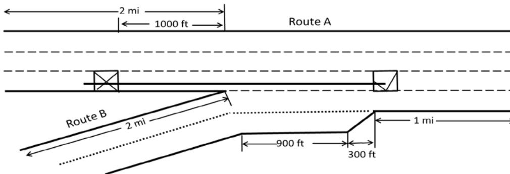
**Figure 52. Illustration. Merging of three- and two-lane freeways (closure on route A).**
