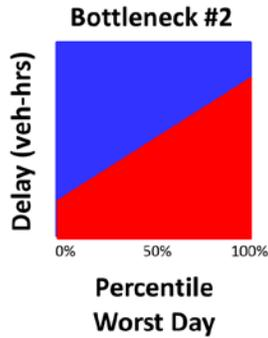
**Figure 22. Graph. ARM illustrating relatively poor bottleneck reliability based on vehicle-hours of delay.**
