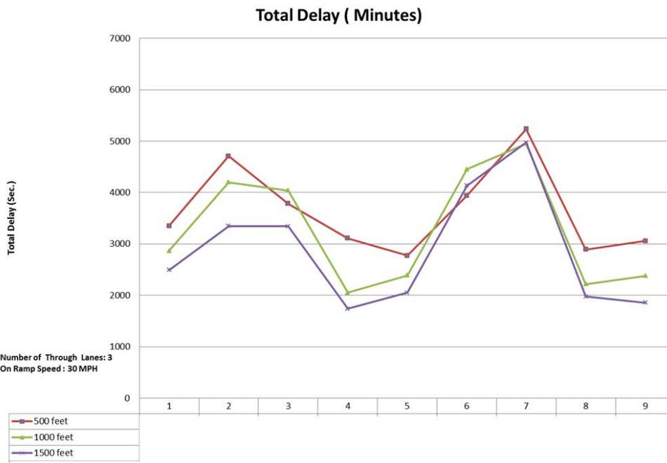
**Figure 67. Graph. Total delay for three mainline lanes and 30-mi/h ramp speed.**
