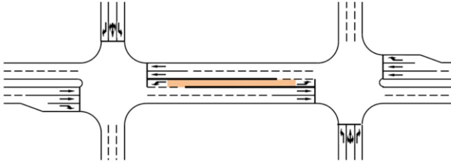
**Figure 83. Illustration. DRLT design for a four-lane road with a single LT lane.**
