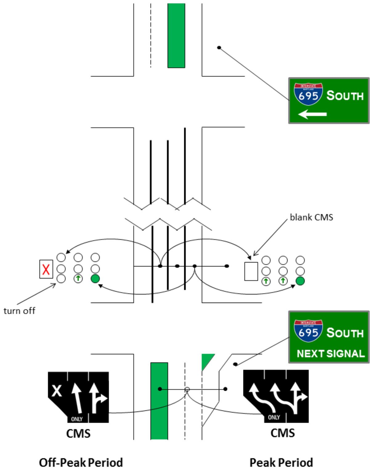
**Figure 89. Illustration. DMSs for dual DRLT lanes during peak and off-peak periods.**
