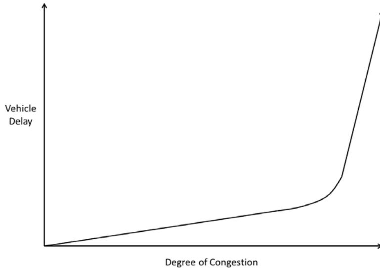
**Figure 2. Graph. Vehicle delay versus degree of traffic congestion.**
