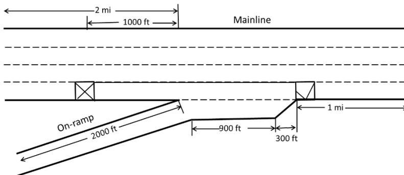
**Figure 55. Illustration. Merging of one-lane ramp and four-lane mainline (closure on mainline).**
