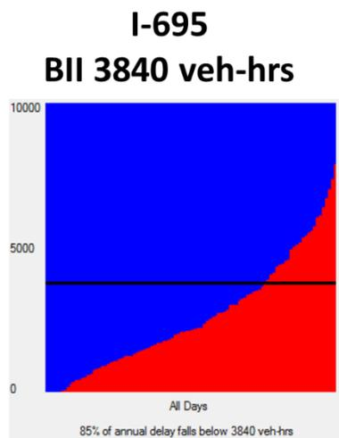
**Figure 23. Graph. Comparison of bottleneck locations based on BII—I-695 example.**
