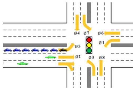
**Figure 30. Illustration. Example of LT congestion prior to DLG.**
