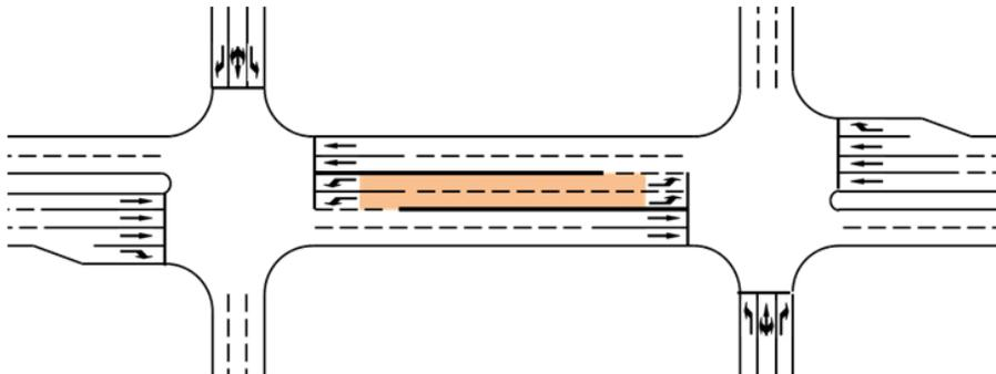
**Figure 85. Illustration. DRLT design for a six-lane road with dual LT lanes.**
