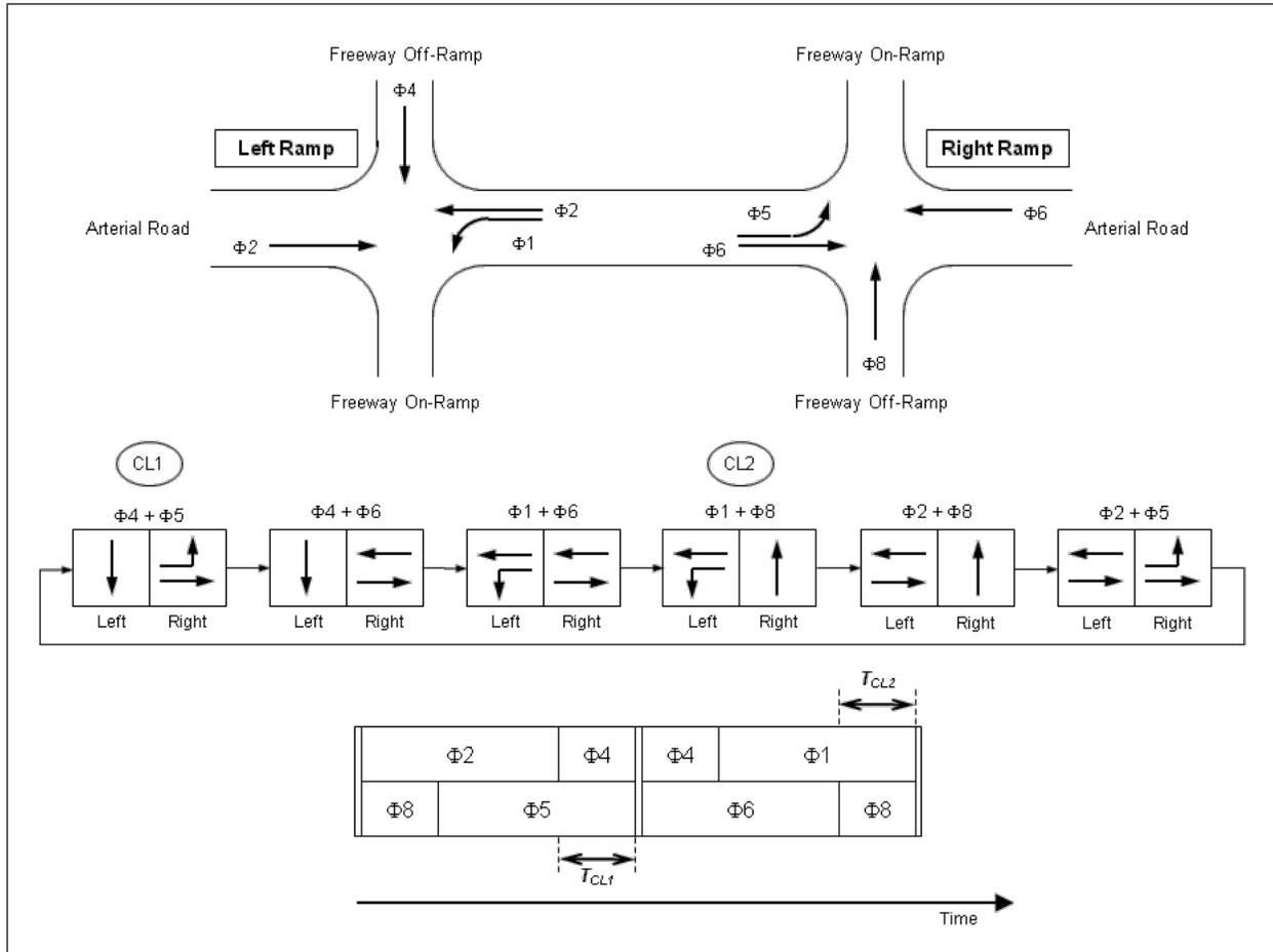
**Figure 90. Illustration. Signal phasing and ring structure for proposed DRLT diamond interchanges.<sup>(76)</sup>**
