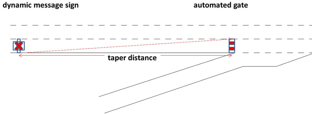
**Figure 62. Illustration. Automated gate option for DMC.**
