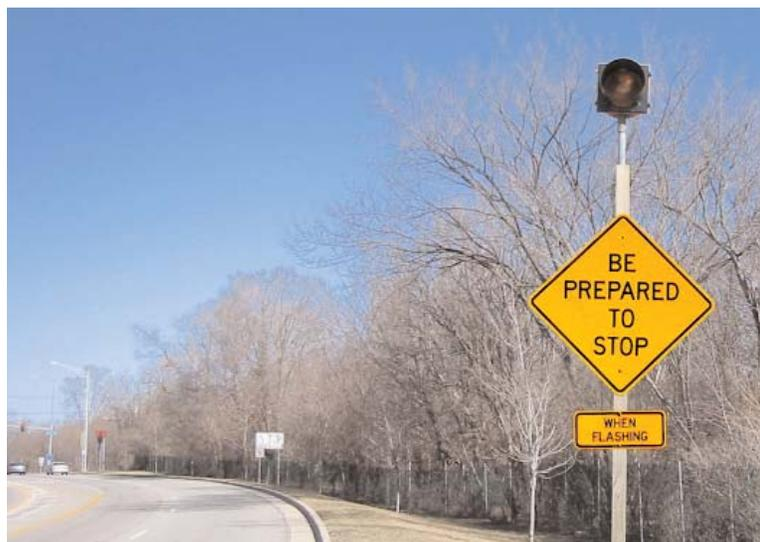
**Figure 92. Photo. Upstream advance warning sign for DRLT.<sup>(80)</sup>**
