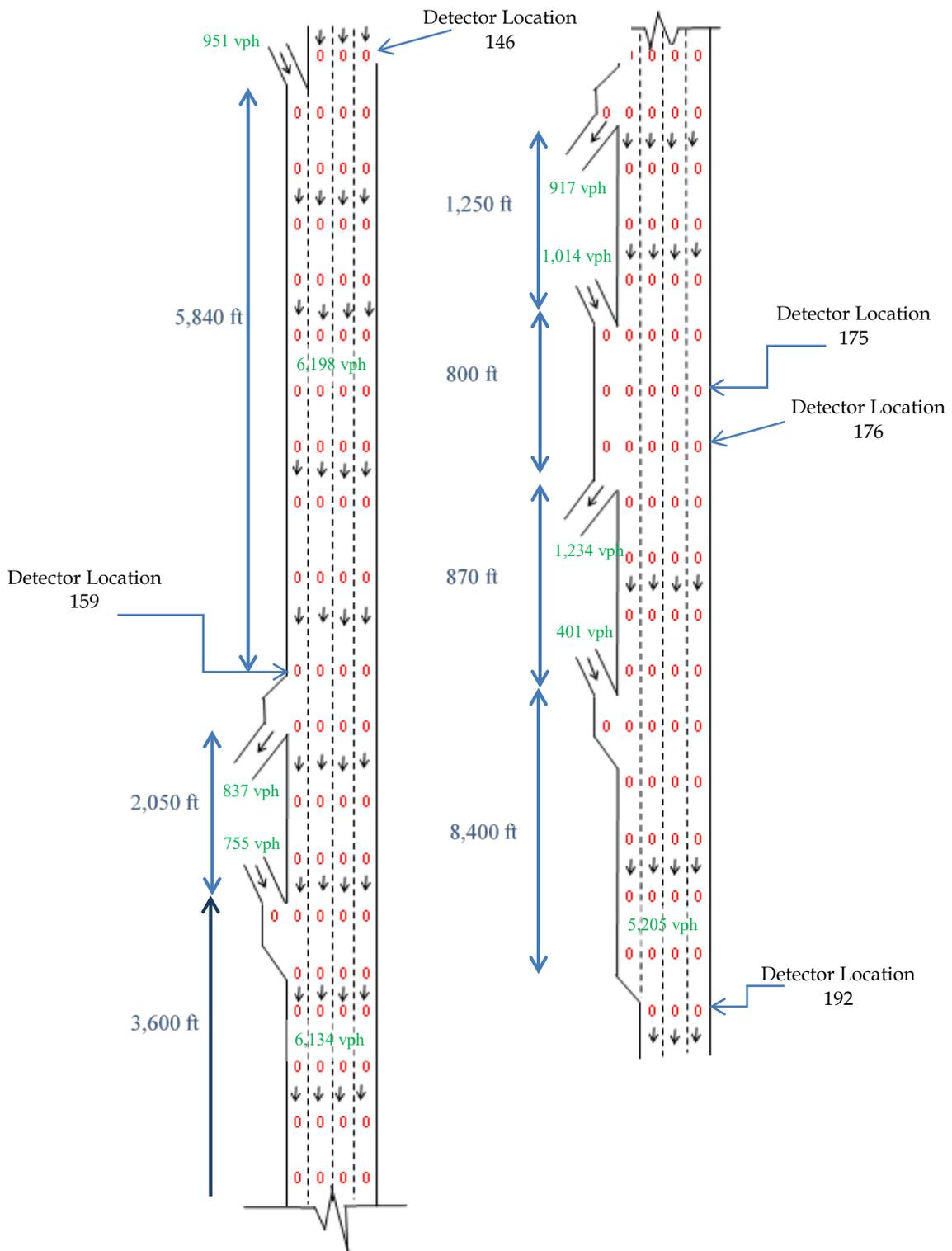
**Figure 73. Illustration. Base year analysis of reducing lane widths to add new lanes.**
