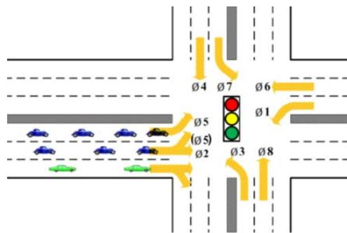
**Figure 31. Illustration. Example of LT congestion after DLG.**
