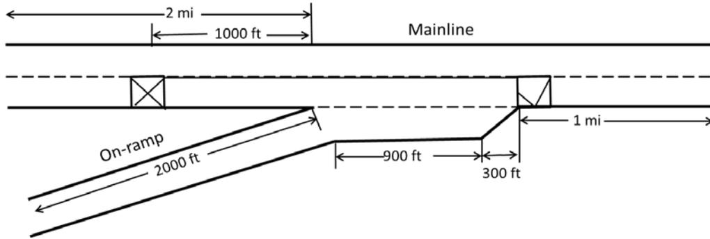
**Figure 53. Illustration. Merging of one-lane ramp and two-lane mainline (closure on mainline).**
