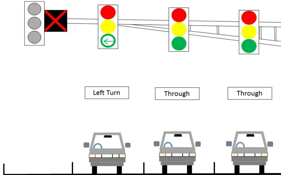
**Figure 107. Illustration. Proposed CLT signalization during off-peak period.**
