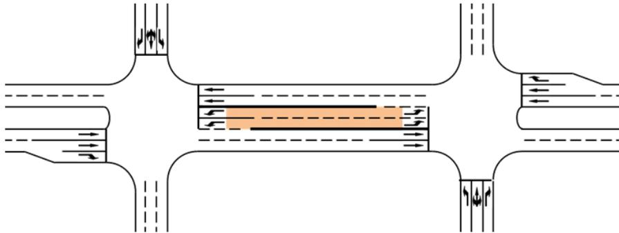
**Figure 84. Illustration. DRLT design for a four-lane road with dual LT lanes.**
