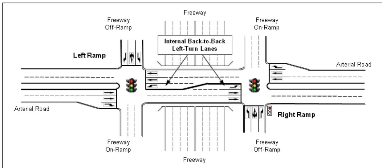
**Figure 78. Illustration. Typical signalized diamond interchange with back-to-back LT lanes.**
