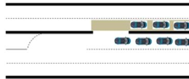
**Figure 100. Illustration. Expected CLT lane utilization under medium LT demand.**
