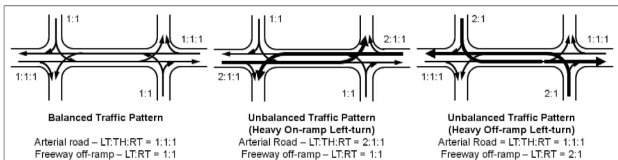
**Figure 80. Illustration. Interchange traffic patterns.**
