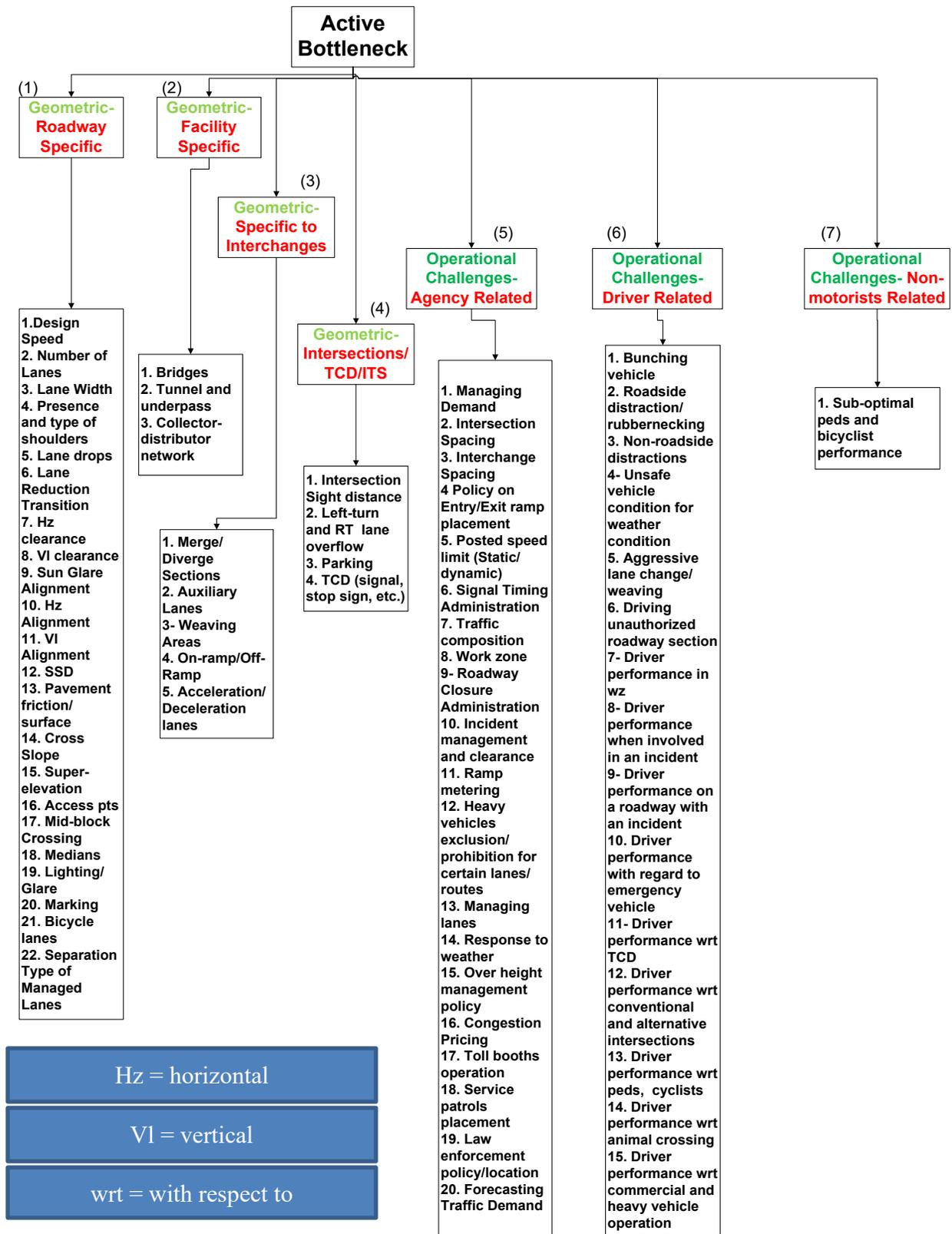
**Figure 29. Flowchart. Framework to identify causes of bottlenecks.**
