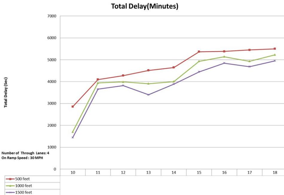
**Figure 69. Graph. Total delay for four mainline lanes and 30-mi/h ramp speed.**
