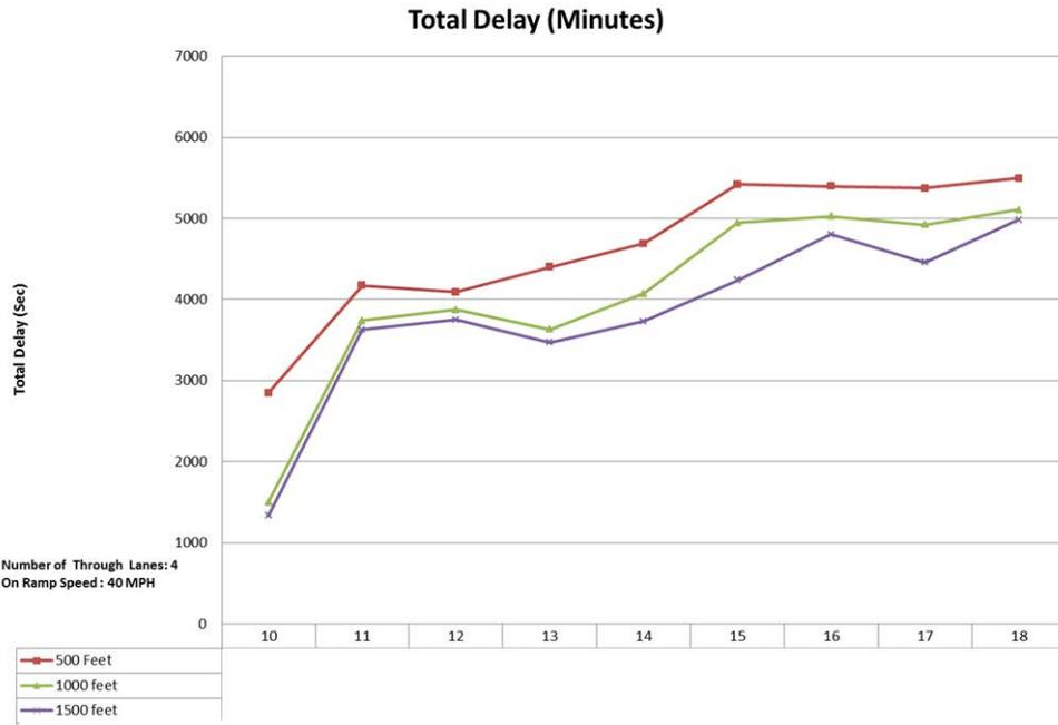
**Figure 68. Graph. Total delay for four mainline lanes and 40-mi/h ramp speed.**
