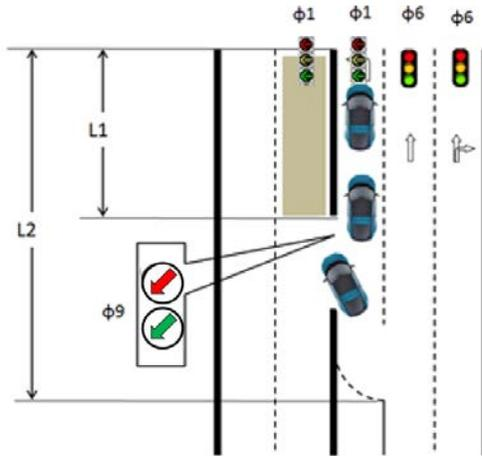
**Figure 98. Illustration. CLT pocket configuration.**
