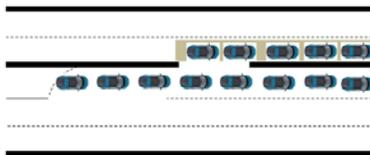
**Figure 101. Illustration. Expected CLT lane utilization under high LT demand.**
