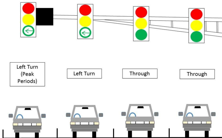
**Figure 106. Illustration. Proposed CLT signalization during peak period.**
