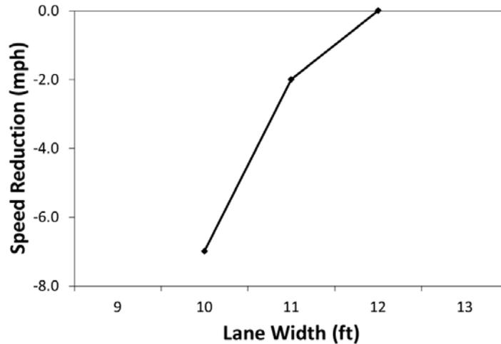
**Figure 75. Graph. Speed reduction as a function of lane width.**
