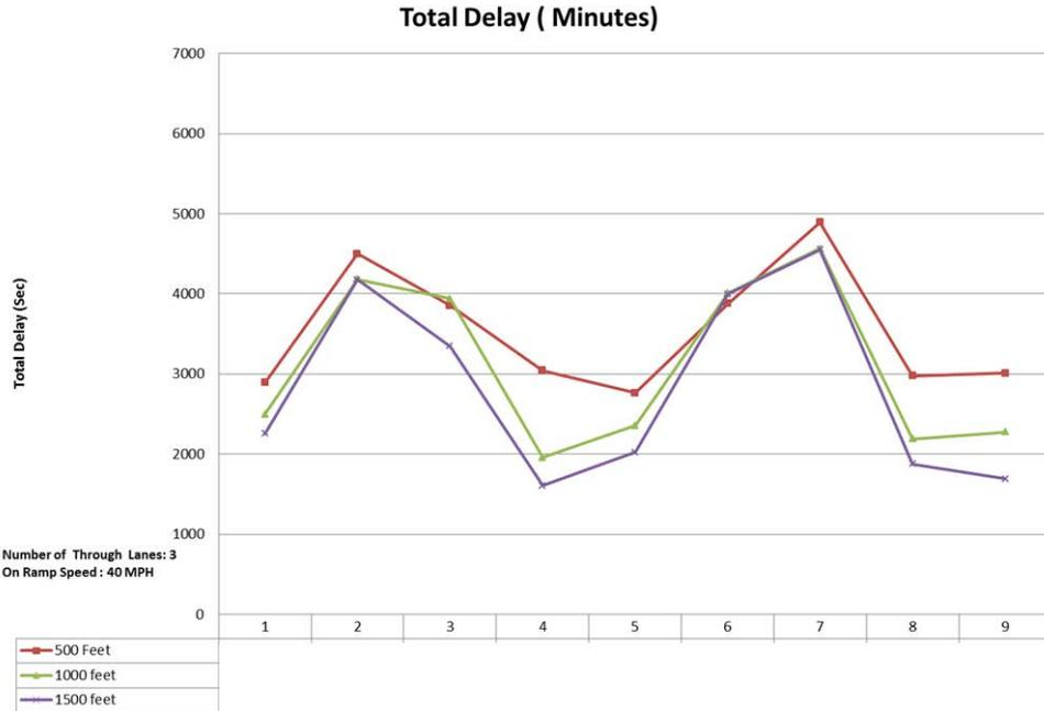
**Figure 66. Graph. Total delay for three mainline lanes and 40-mi/h ramp speed.**
