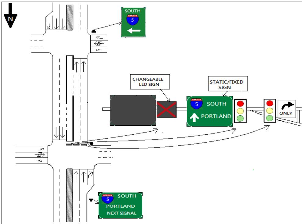
Figure 88. Illustration. Proposed single-lane DRLT signalization during red phases for all periods.
