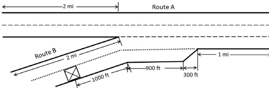
**Figure 49. Illustration. Merging of multiple two-lane freeways (closure on route B).**
