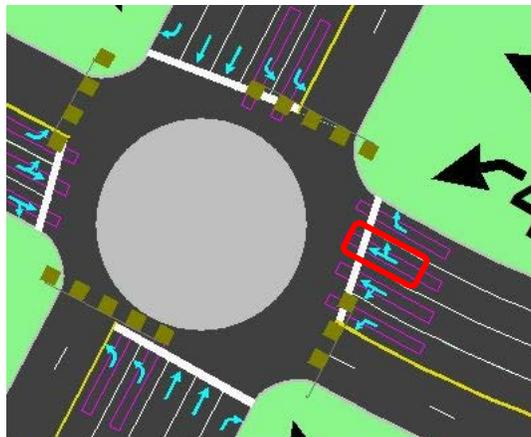
**Figure 42. Illustration. Lane assignment after DLG for case study 1.**
