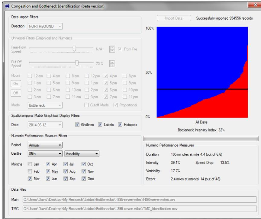
**Figure 17. Screenshot. CBI tool with ARM (upper right) and speed drop (lower right).**
