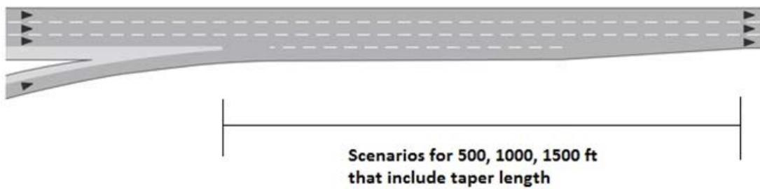
**Figure 64. Illustration. Acceleration lane length schematic (three-lane configuration).**
