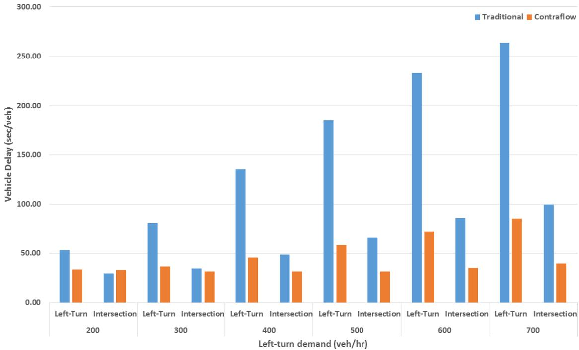
**Figure 96. Graph. Delay reductions due to CLT at various LT demand levels.**
