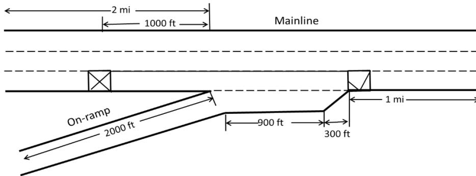
**Figure 54. Illustration. Merging of one-lane ramp and three-lane mainline (closure on mainline).**
