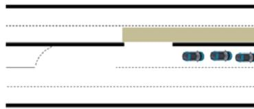
**Figure 99. Illustration. Expected CLT lane utilization under low LT demand.**
