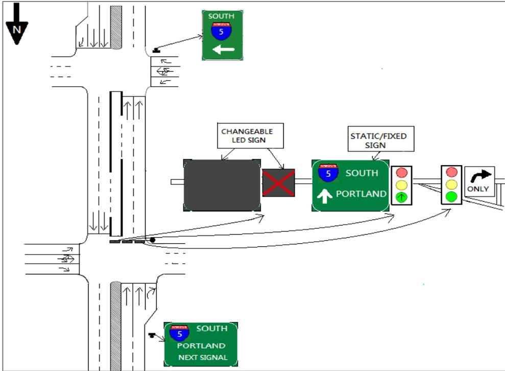
Figure 87. Illustration. Proposed single-lane DRLT signalization during off-peak-period green phases.
