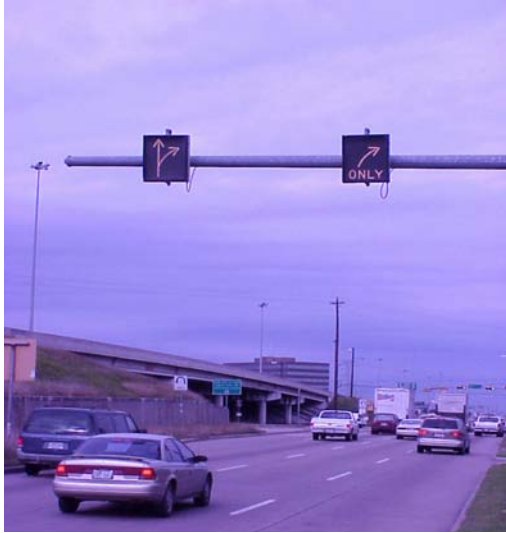
Figure 10. Photo. Dynamic lane assignment on an arterial.
