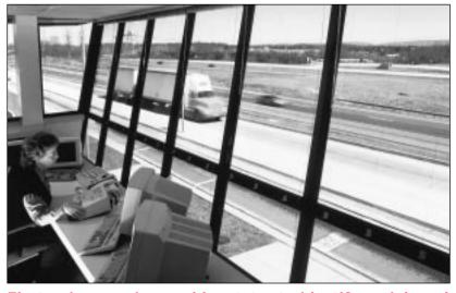
Electronic screening enables states to identify, weigh and check safety and credentials for trucks at highway speeds. Drivers of safe and legal trucks are electronically notified of their status and directed past the station.
