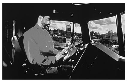
On-board computers and satellite tracking systems can improve communications between dispatchers and drivers. This translates into more efficient equipment utilization, better routing schemes, higher driver job satisfaction, and improved customer service.
