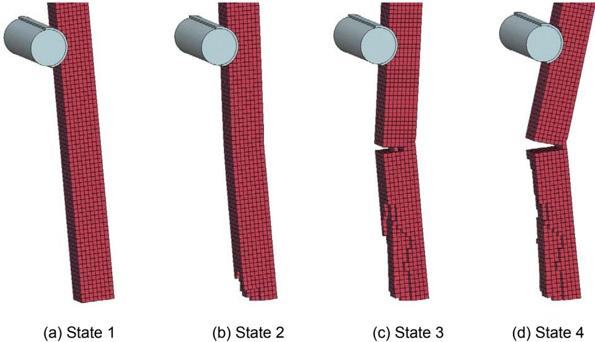
**Figure 92. Element vaporization at bottom of post.**
