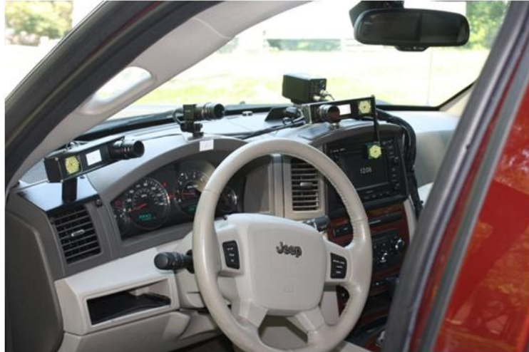
Figure 16. Photo. Eye-tracking system with three dash-mounted cameras and two infrared flashers.
