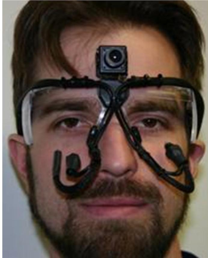
**Figure 61. Photo. MPI system performance experiment—eye-tracker goggles.**
