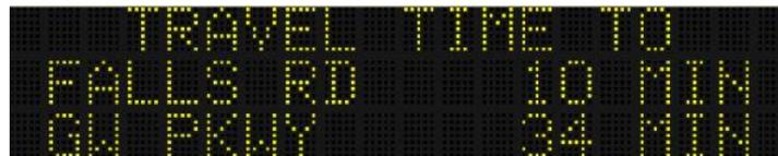
**Figure 61. Illustration. Example of a sign demonstrating recommended capitalization and abbreviation.**
