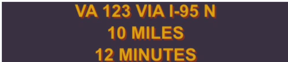
**Figure 34. Illustration. Example of information shown on the travel time display.**
