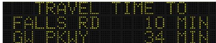
**Figure 59. Illustration. Example of a sign with left and right justifications.**
