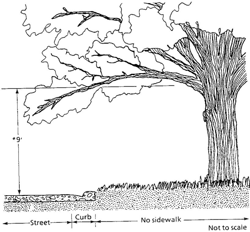
Branches should be trimmed so that there is 9' of clear space above the pavement (street and/or sidewalk).
