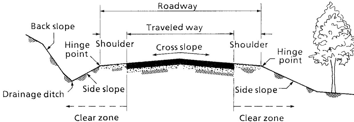
**Hinge Point** Point where the slope rate changes.
