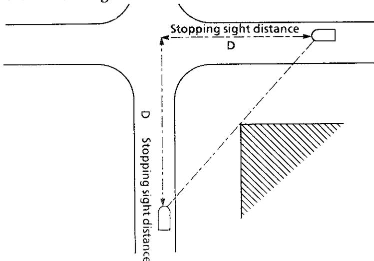
At intersections with no stop signs (or with stop signs only at the cross street), drivers from all (both) directions need to be able to see oncoming traffic soon enough to be able to stop. This stopping sight distance is distance D in the drawing above. The table below lists the stopping sight distance needed for different speed limits on a street.
