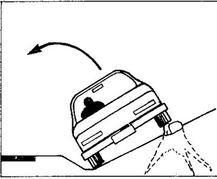
Rolling of the vehicle occurs when the wheel or the under-carriage rides up on a stump on a slope. Cutting a stump off as close to flush with the slope as possible minimizes the roll over danger.
