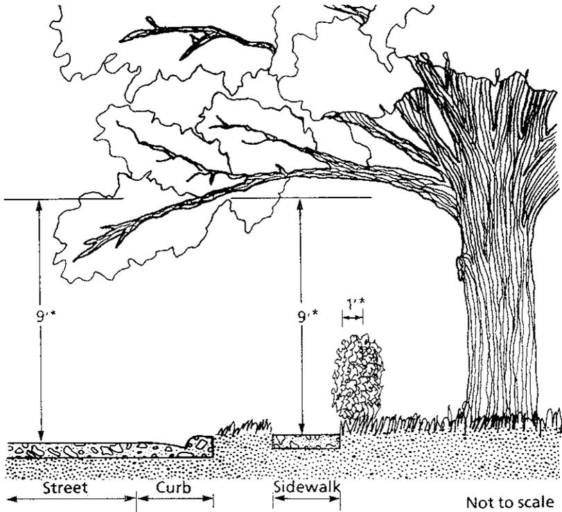
Branches should be trimmed so that there is 9' of clear space above the pavement (street and/or sidewalk). Bushes obstructing sidewalks should be trimmed back so that there is 1' clearance between the bush and the sidewalk.
