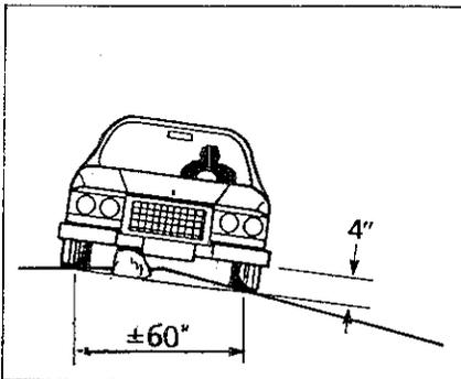
Snagging occurs when a vehicle undercarriage catches on a stump or other object. Generally, any stump higher than 4 inches above the surrounding ground can cause snagging.
