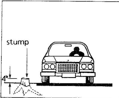
Small diameter trees should be cut off no more than 4 inches from the ground. Large diameter trees should be cut flush with the ground. Trees of any size growing on a slope should be cut flush with the ground.
