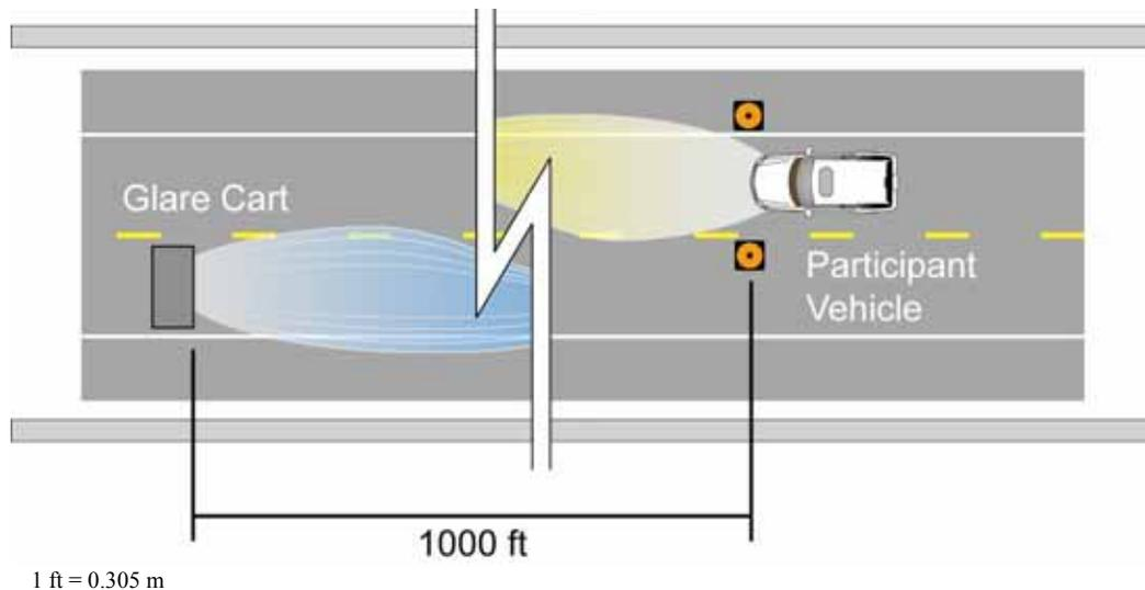
**Figure 8. Diagram. Plan view of the participant vehicle at the start point in the discomfort glare portion.**
