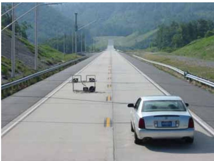
**Figure 6. Photo. Glare cart and experimental vehicle on the Smart Road.**
