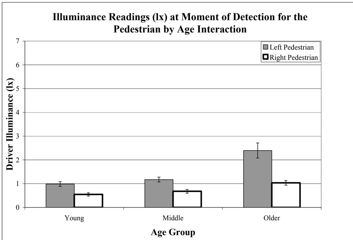
**Figure 16. Bar graph. Mean illuminance readings (lx) at moment of detection for the Pedestrian by Age interaction.**
