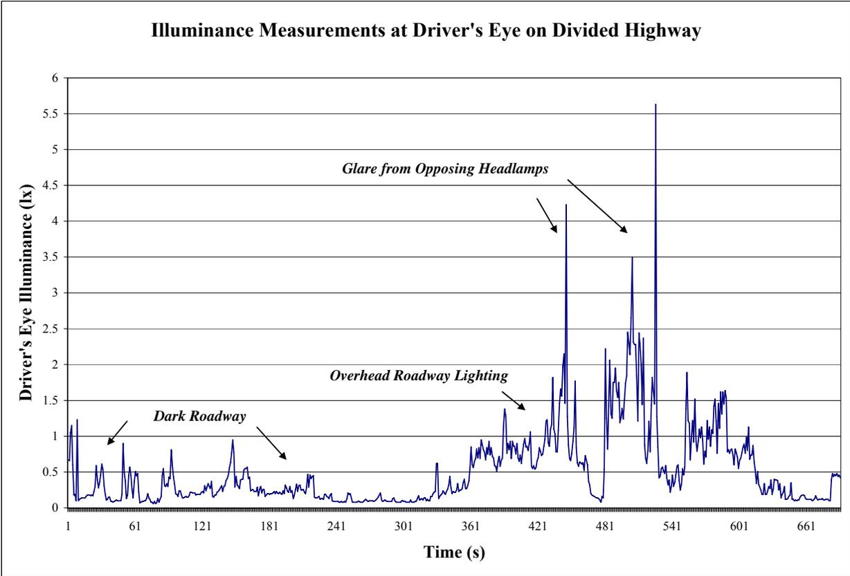
Figure 2. Line graph. Illuminance readings taken on a divided highway at night with and without overhead lighting and glare.
