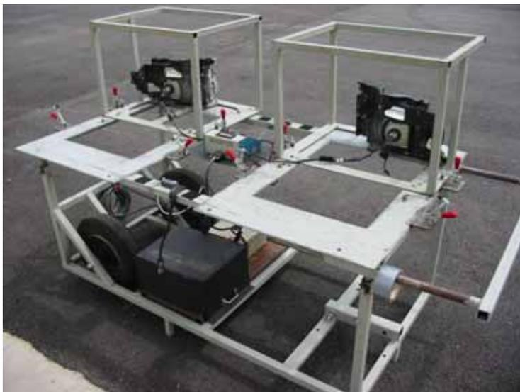
**Figure 5. Photo. Back view of glare cart with halogen VESs (low/narrow) mounted.**
