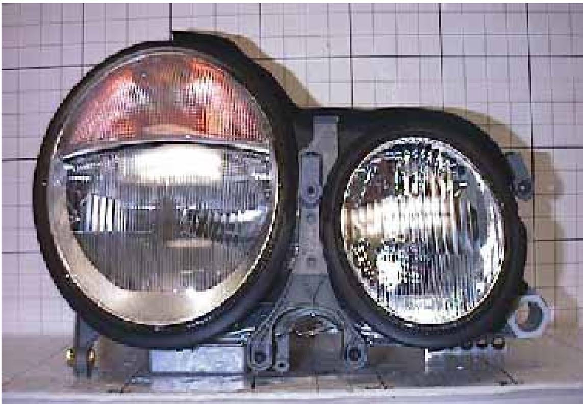
**Figure 22. Photo. Front view of HID 1 headlamp (high/narrow).**
