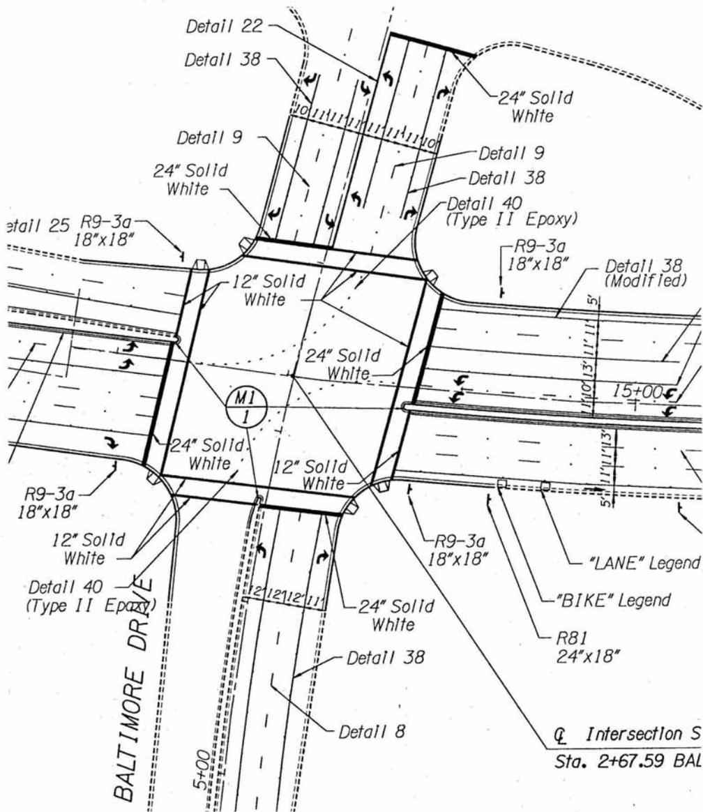
**Figure 10-17. Illustration. Example signing and marking plan for SR 8 by Fletcher Parkway Construction Plans, La Mesa, CA.**
