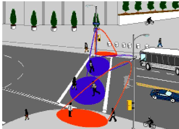
**Figure 10-14. Example of a microwave detector system.**
