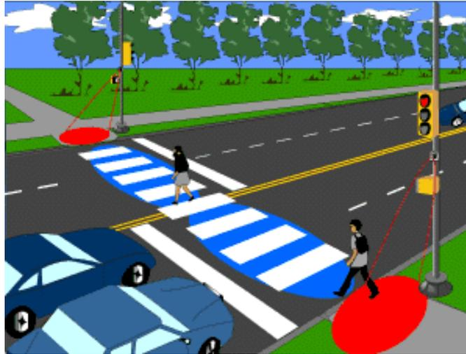
**Figure 10-15. Illustration. Example of an infrared detector system.**
