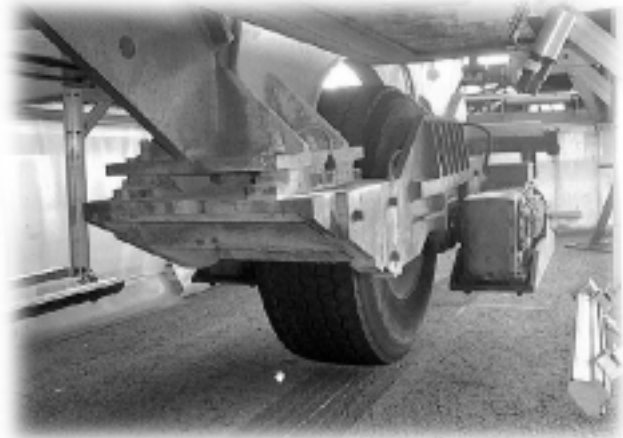
Close-up view of the ALF single wheel and tire.
